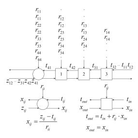
(a) 1-D structure. The boundary cell is complex-valued subtraction and division, and internal cells are complex-valued addition.
