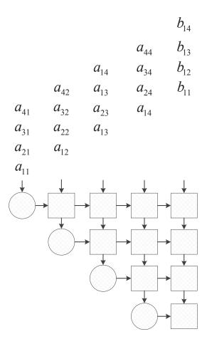
Figure 3.4. Conventional systolic array QRD for solving As = b.
