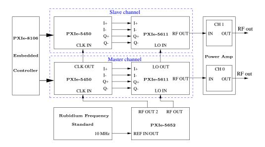
(a) Structure of the 2-channel transmitter. The power amplifiers were NI-5691 Dual RF Amplifier or RF Bay's MPA10-40. If 4-channel transmitter was desired, then two more channels were added as slave channels with two additional PXIe-5450 I/Q Signal Generators and two PXIe-5611 Modulators.
