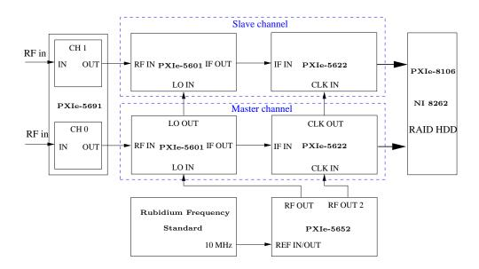
(b) Structure of the 2-channel receiver. If 4-channel receiver was used, then two additional channels were added as slave channels with two PXIe-5622 IF Digitizers and two PXIe-5601 RF Down-convertors, plus another PXIe-5691 RF Amplifier serving as the low noise amplifier.
