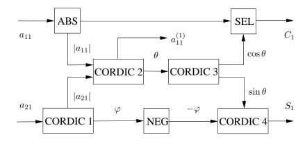
Figure 3.1. The block diagram of qr\_sub module.
