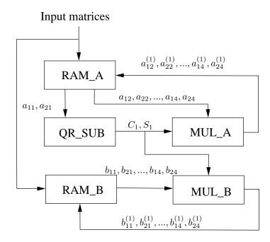
Figure 3.3. Data flow diagram of the proposed QRD scheme.
