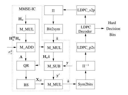
Figure 3.1. Block diagram of the implemented MMSE-IC turbo detector.
