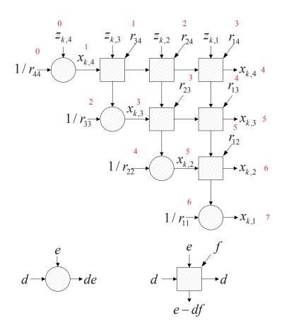
Figure 3.3. 2-D systolic arrays for back substitution.
