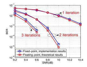
Figure 5.2. The BER performance versus SNR.
