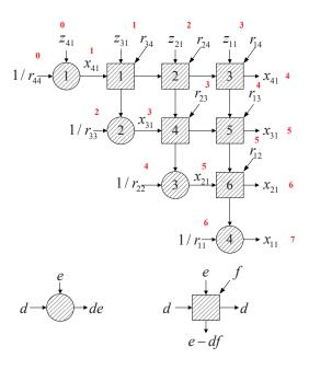
(b) 2-D structure. The boundary cells are multipliers of a real number with a complex number, and internal cells are complex-valued multiplication and subtraction. The numbers in boldface denote the input and output timing in processing cycle count.
