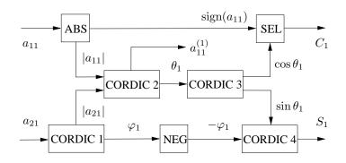
Figure 3.2. The block diagram of QR\_SUB module.
