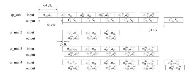
Figure 3.2. Timing control for 4-CORDIC QRD.
