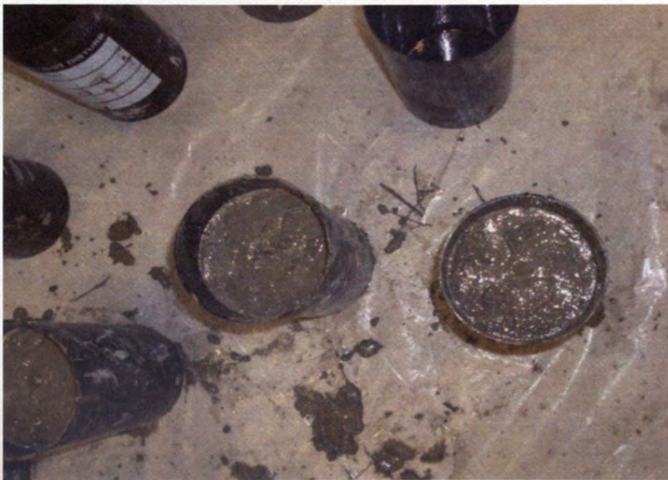
Figure 3.13 – Wet Concrete in Cylinder Molds
