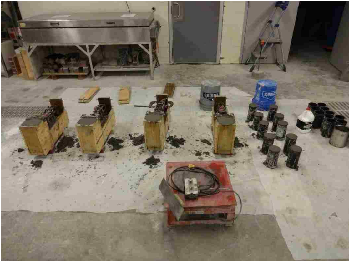
Figure 3.14. Completed first lift of cold-joint specimens
