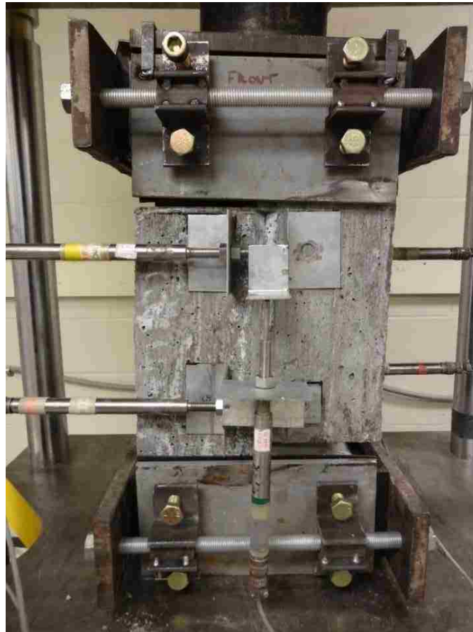
Figure 3.20. LVDT configuration to measure slip and dilation
