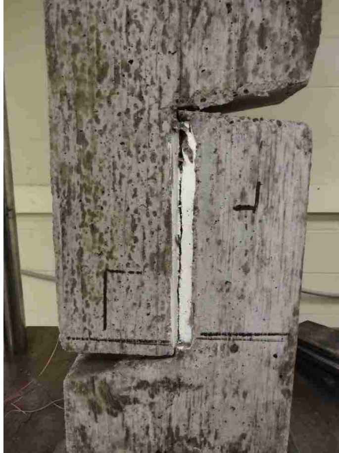
Figure 3.22. Typical specimen failed in shear along the intended shear plane
