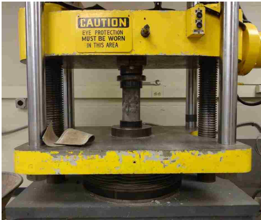
Figure 3.6. Compressive strength test set-up
