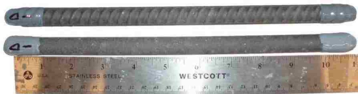
Figure 4.1: A typical smooth and deformed salt spray specimen prior to testing.
