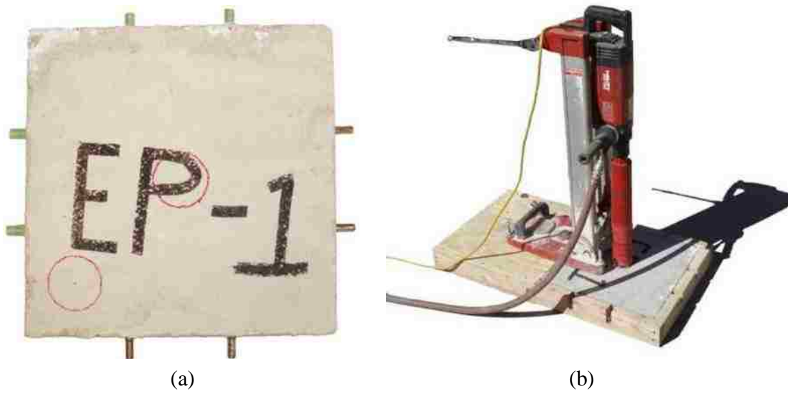
Figure 3.8: Coring of a ponding specimen. (a) Coring locations. (b) Equipment used.
