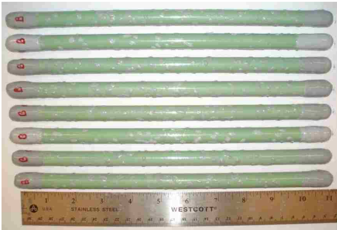
Figure B - 21: Backside of the smooth epoxy-coated salt spray specimens after testing.
