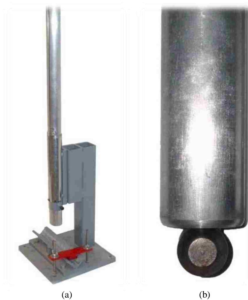
Figure 3.2: Apparatus used to damage coated bars. (a) Overall view. (b) Tip of the tup aligned within the hollow aluminum tube.
