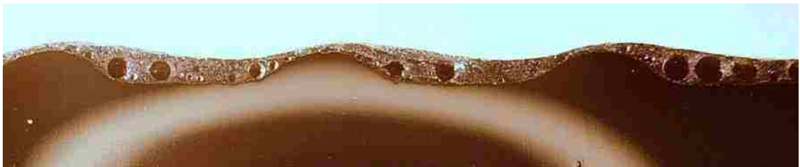
Figure 4.14: Cross-sectional views of the pure enamel coating along smooth and deformed specimens. (a) A longitudinal view of the pure enamel coating distributed along a deformed specimen that had performed well during the test.
