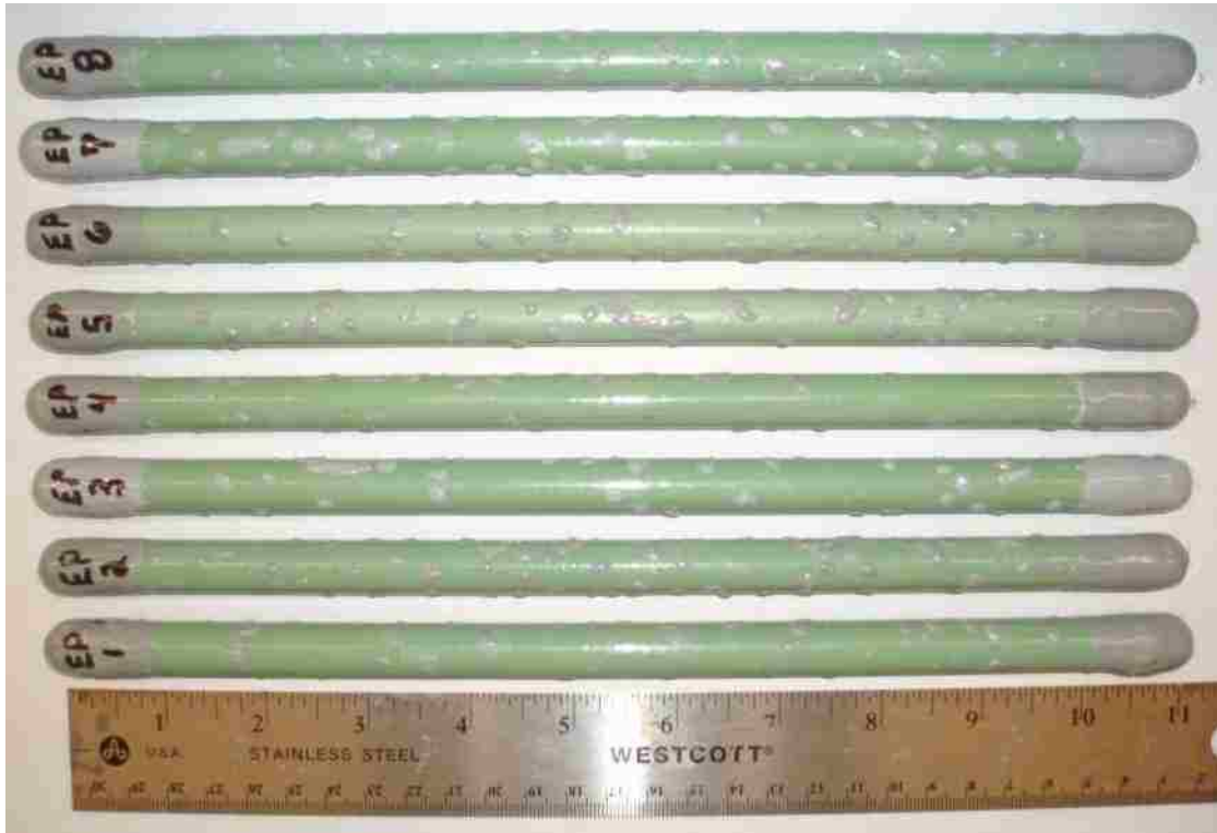
Figure B - 20: Front side of the smooth epoxy-coated salt spray specimens after testing.
