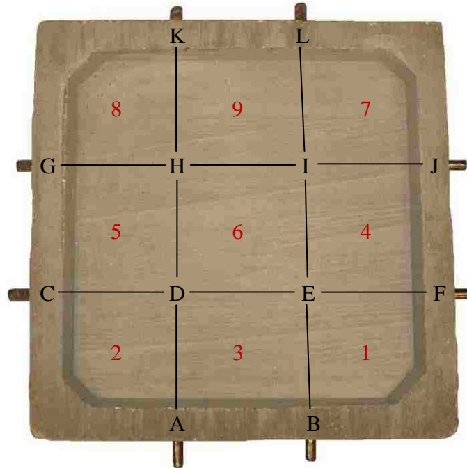
Figure 3.10: The nine sections of a ponding specimen.
