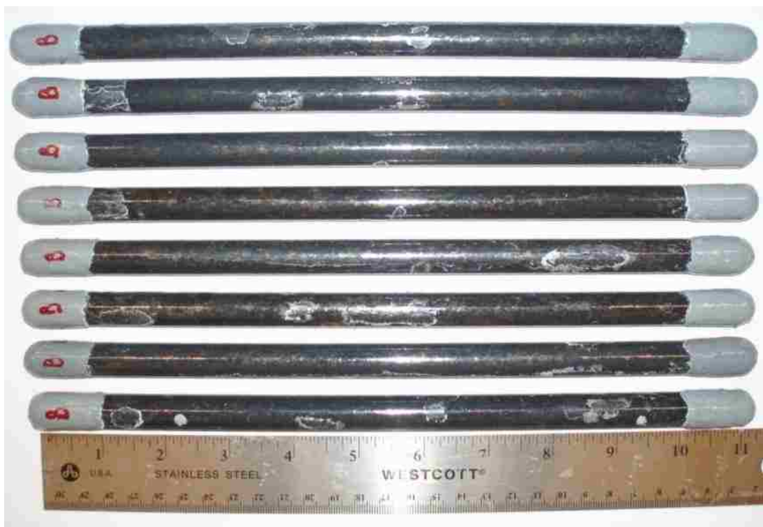
Figure B - 15: Backside of the smooth pure enamel-coated salt spray specimens after testing.
