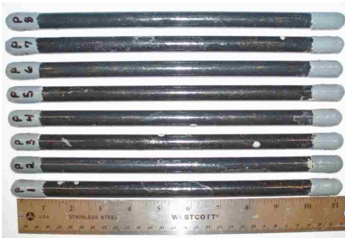
Figure B - 14: Front side of the smooth pure enamel-coated salt spray specimens after testing.
