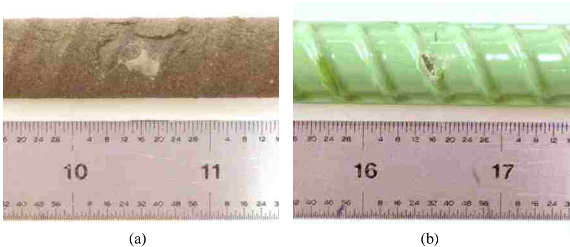
Figure 3.3: Representative view of an average intentionally damaged area along the two tested coatings. (a) 50/50 enamel. (b) epoxy.
