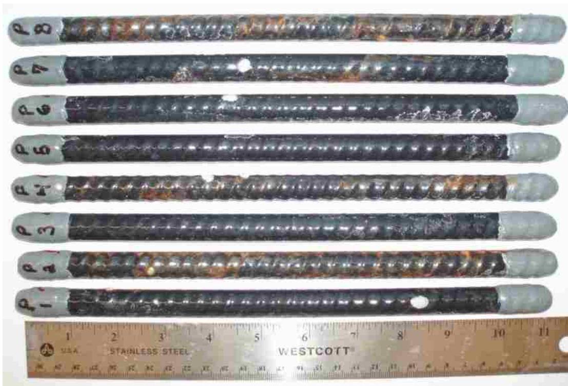
Figure B - 16: Front side of the deformed pure enamel-coated salt spray specimens after testing.
