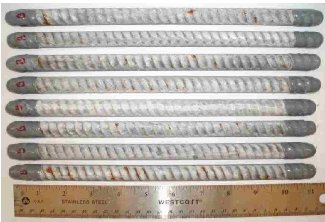
Figure B - 11: Backside of the deformed double enamel-coated salt spray specimens after testing.
