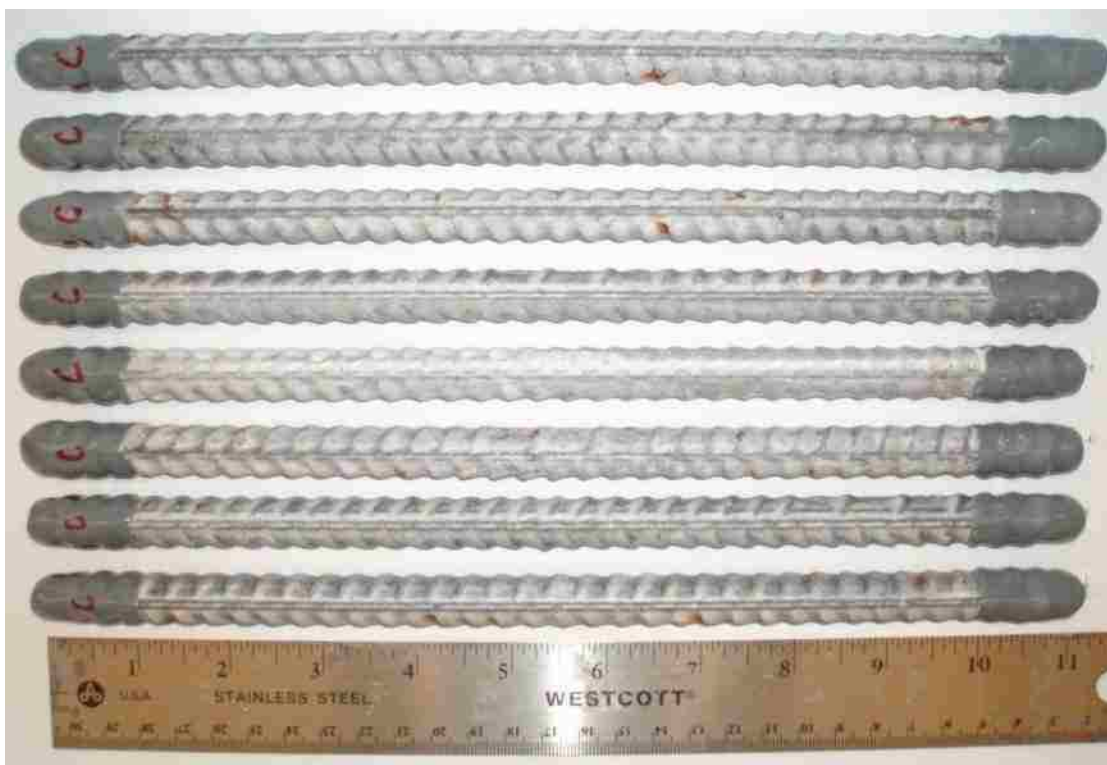
Figure B - 13: Left side of the deformed double enamel-coated salt spray specimens after testing.
