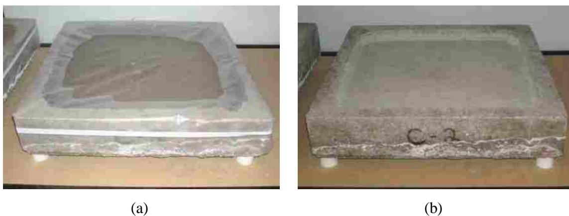
Figure 3.5: Typical ponding specimen during either the wet or dry phase of testing. (a) Wet phase. (b) Dry phase.
