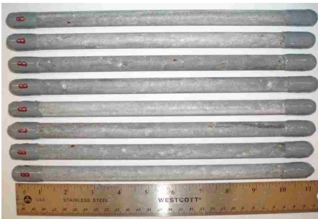
Figure B - 9: Backside of the smooth double enamel-coated salt spray specimens after testing.
