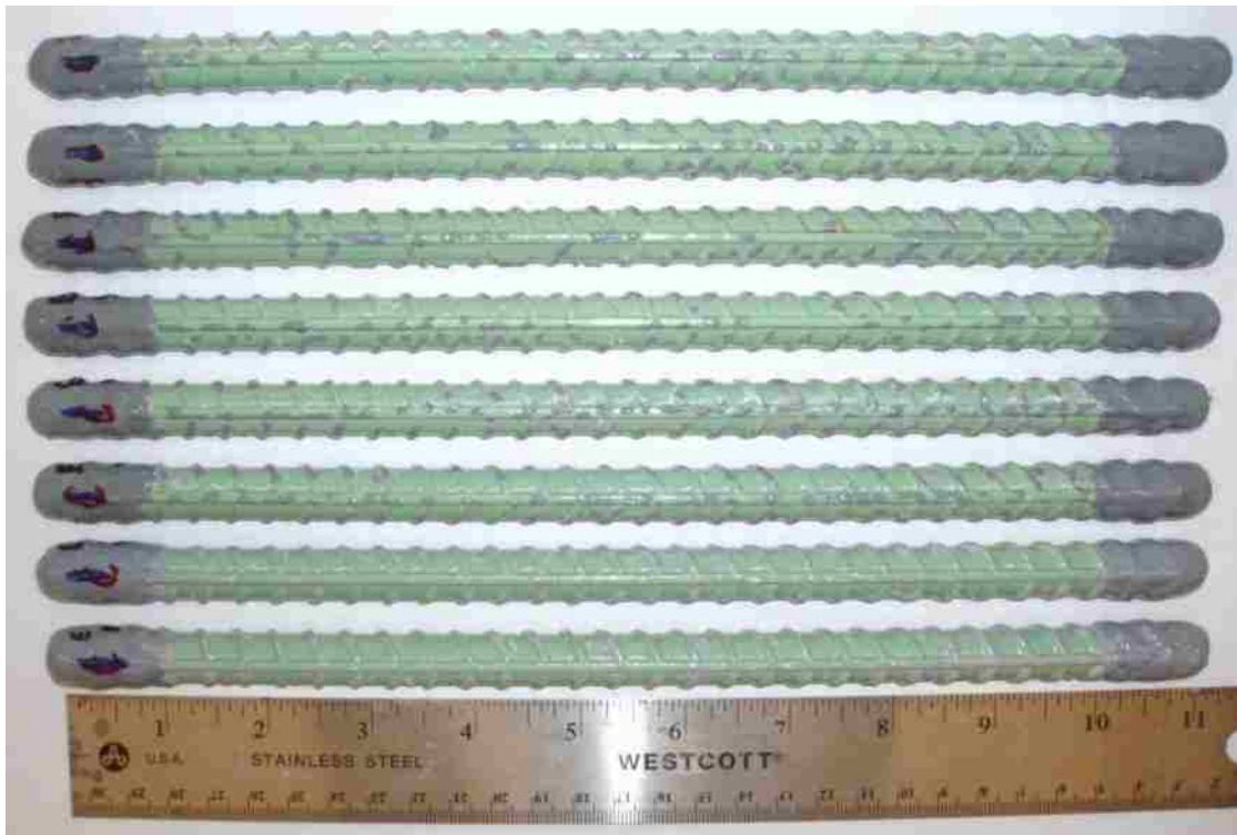
Figure B - 25: Left side of the deformed epoxy-coated salt spray specimens after testing.
