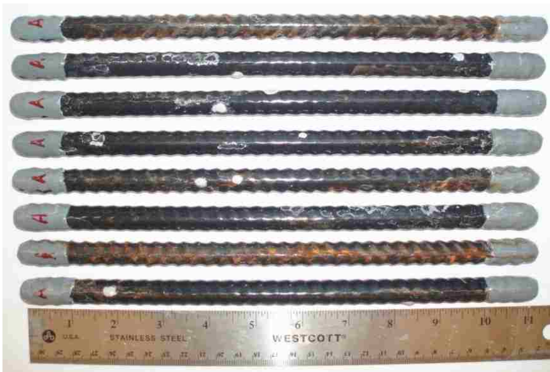
Figure B - 18: Right side of the deformed pure enamel-coated salt spray specimens after testing.
