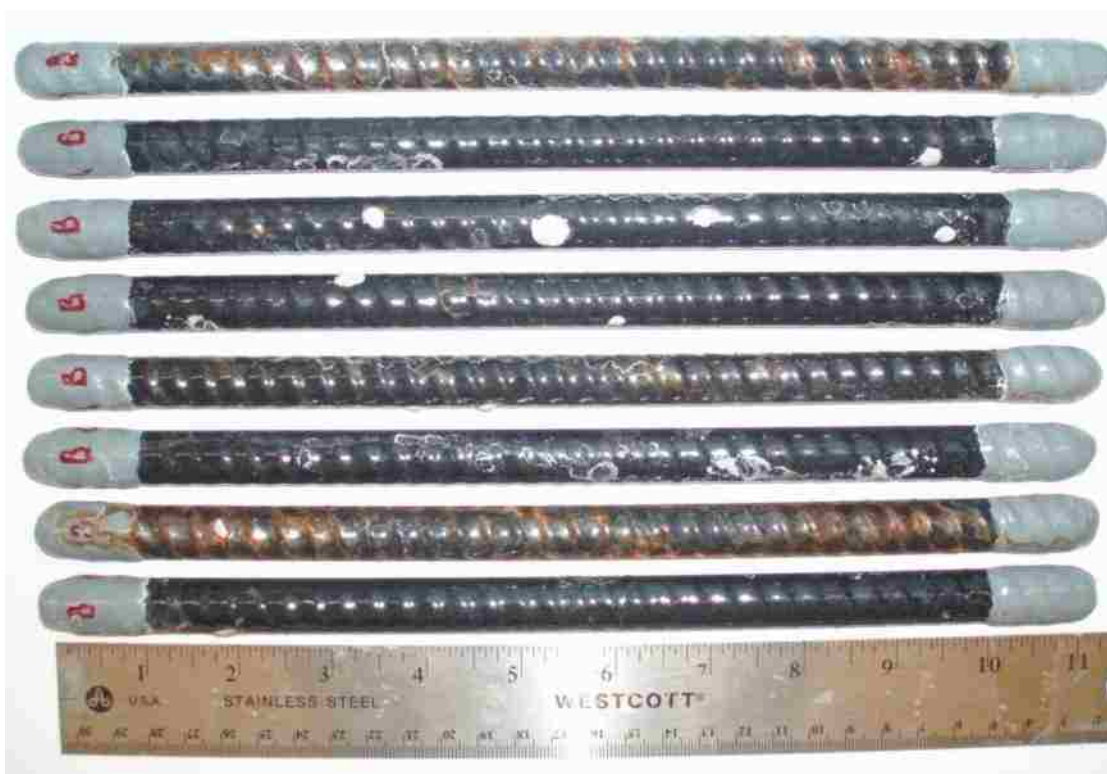
Figure B - 17: Backside of the deformed pure enamel-coated salt spray specimens after testing.
