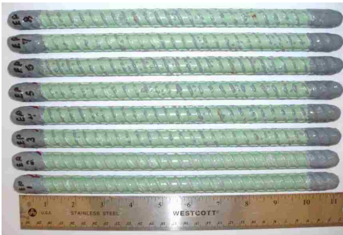
Figure B - 22: Front side of the deformed epoxy-coated salt spray specimens after testing.
