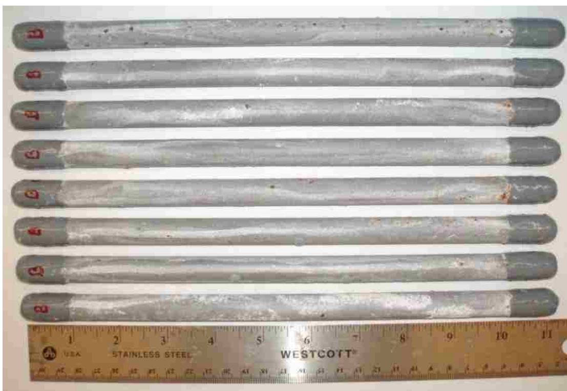
Figure B - 3: Backside of the smooth 50/50 enamel-coated salt spray specimens after testing.
