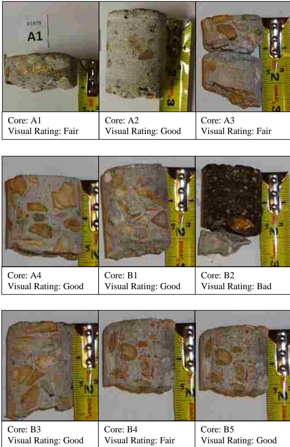
Figure B.1. Bridge A1479 Core Photographs
