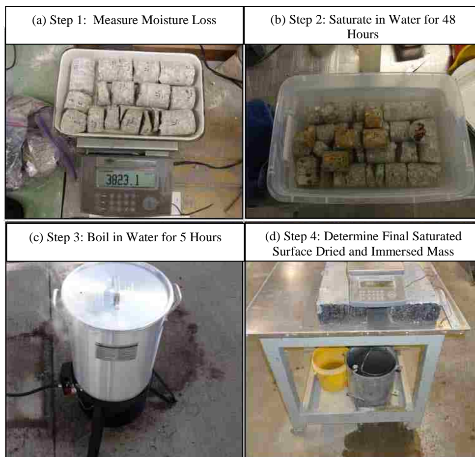
Figure 3.8. Process of Determining Volume of Permeable Pores
