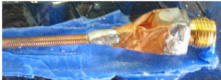
Figure 4.2. Die-cut crack sensor
