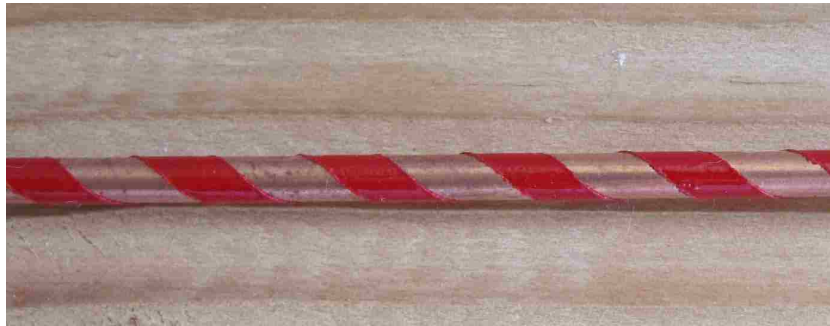
Figure 6.9. Corrosion resistant helical paints over a coaxial cable sensor
