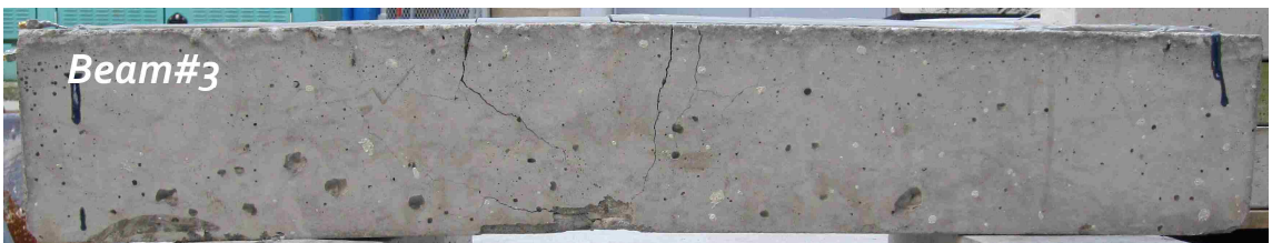
Figure A.2. Beam # 3_ Sika Grout 212_ Hold Tight ® 102
