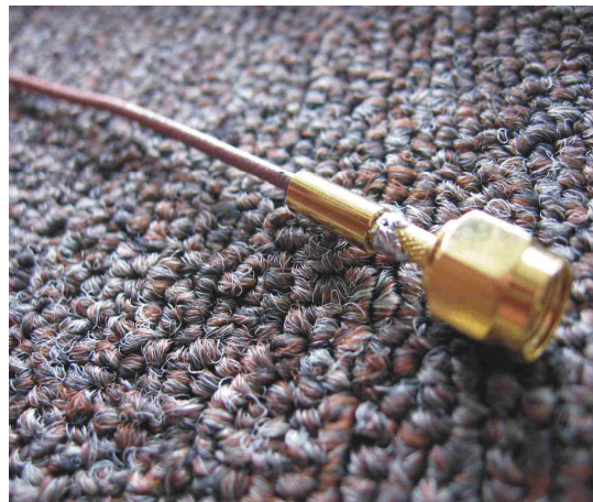
Figure 4.1. Miniaturized crack sensor
