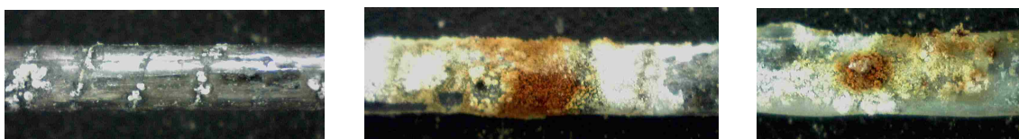
Figure 6.5. Normalized signatures and images of the sensor placed into 5% NaCl solution
