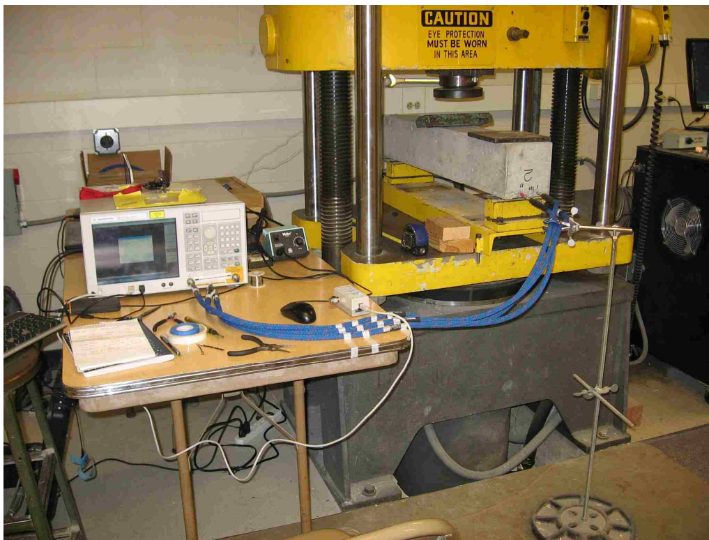
Figure 4.7. Three-point bending test setup
