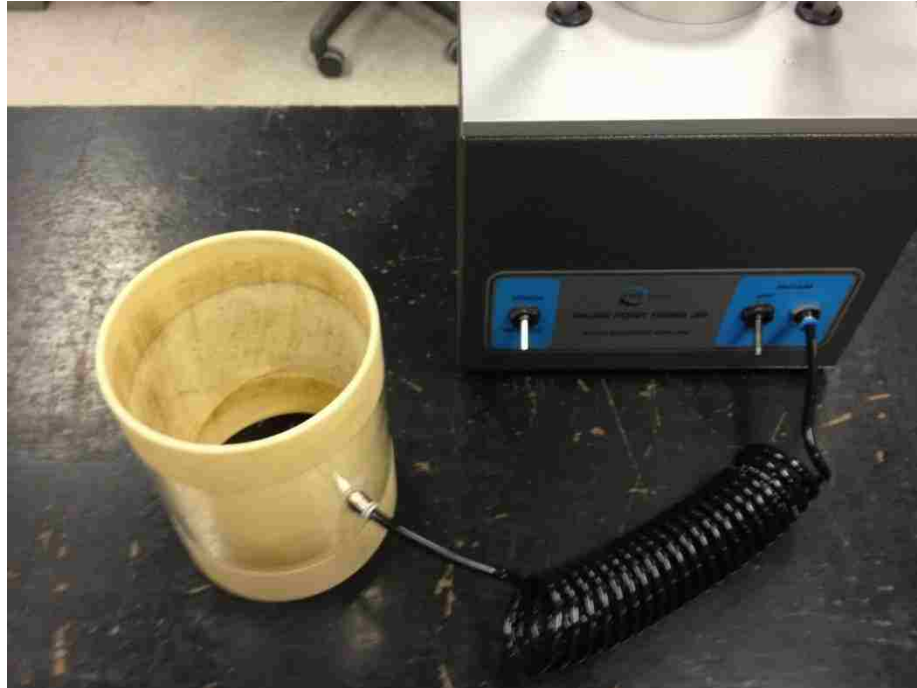
Figure 1 – Membrane Over Collar with Vacuum Applied
