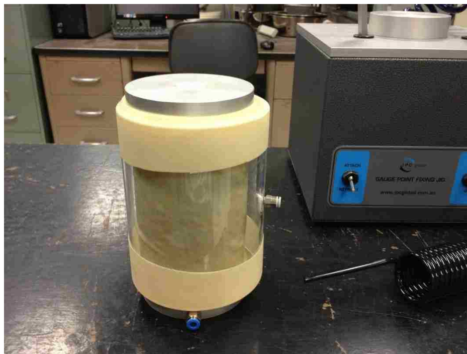
Figure 2 – Collar/Membrane Over Specimen with Vacuum Released
