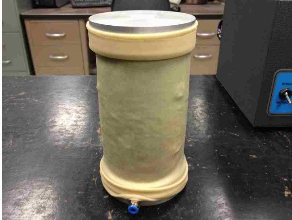
Figure 3 – Excess Membrane Folded Over Plates
