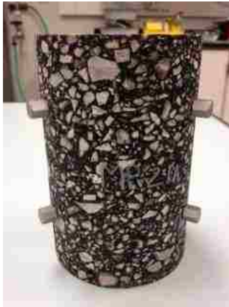
Figure 3 - Specimen with Gauge Points Attached
