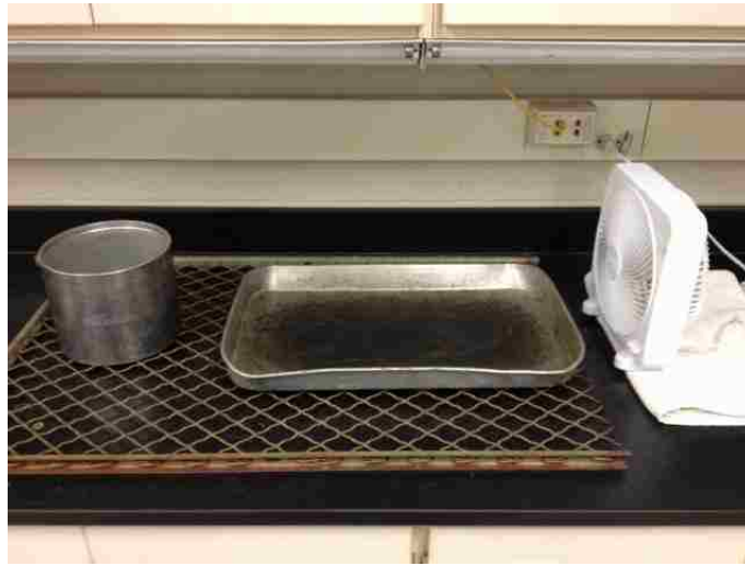
Figure 3.5 - Pycnometer; Cooling Pan and Fan
