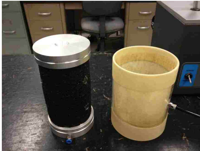
Figure 3.52 - Specimen with Platens and Vacuum Collar with Latex Membrane
