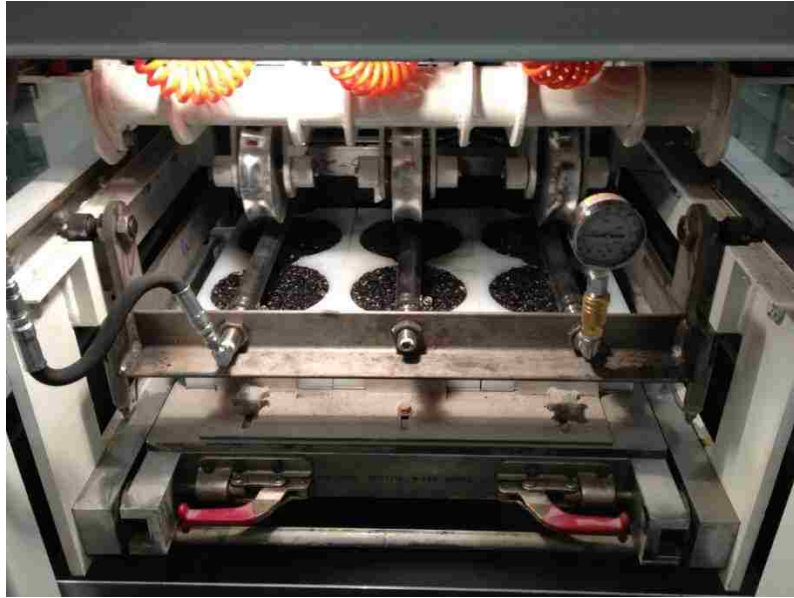
Figure 3.20 - APA Rut Test Setup
