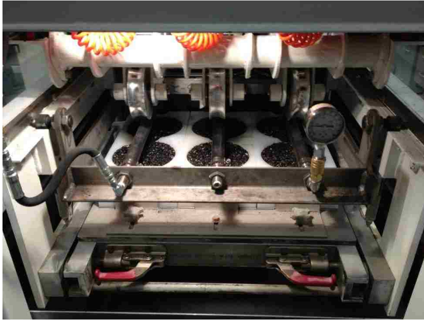
Figure 6 – Hose Carriage and Rutting Specimens
