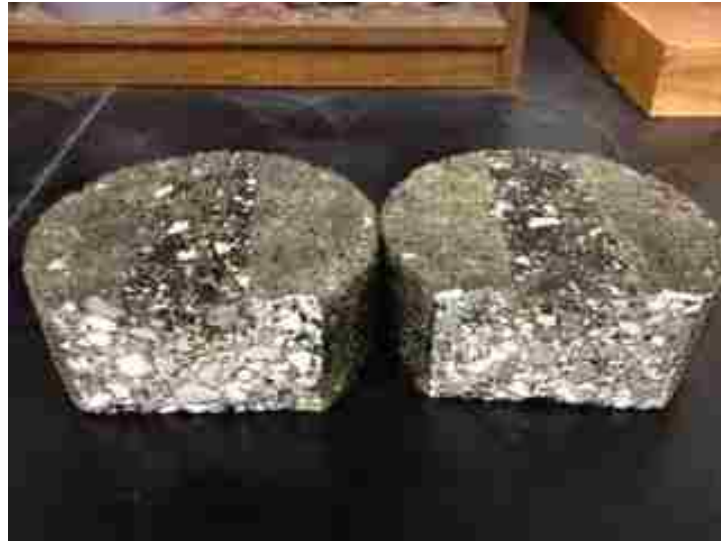
Figure 7 - Cut Side on Hamburg Specimens
