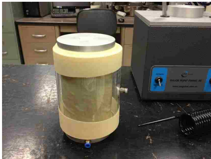
Figure 3.53 - Latex Membrane Installed Over Specimen and Platens
