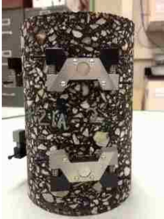
Figure 6 - Clips attached to Gauge Points
