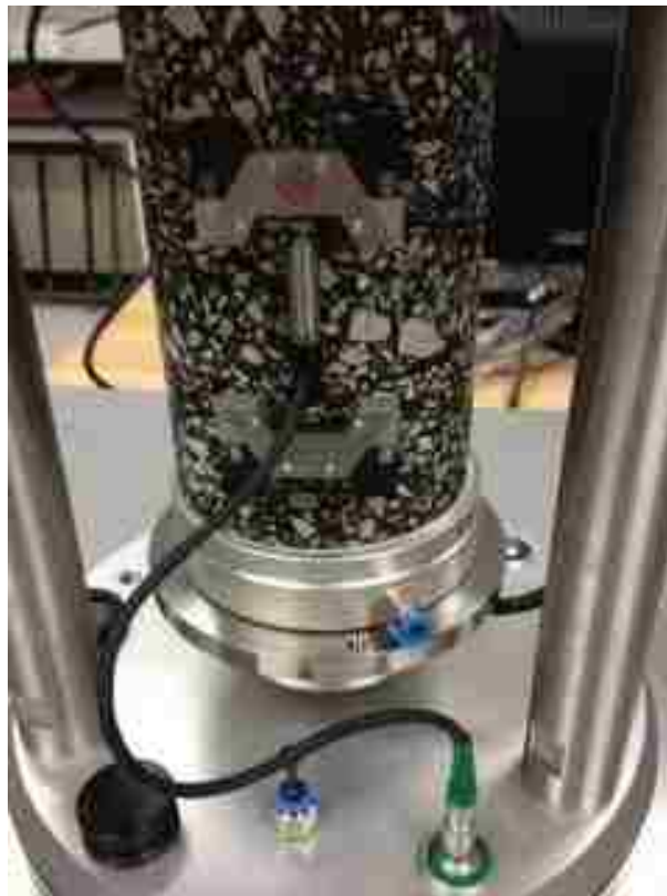
Figure 3.50 - Specimen Loaded Into Test Chamber with LVDTs Attached
