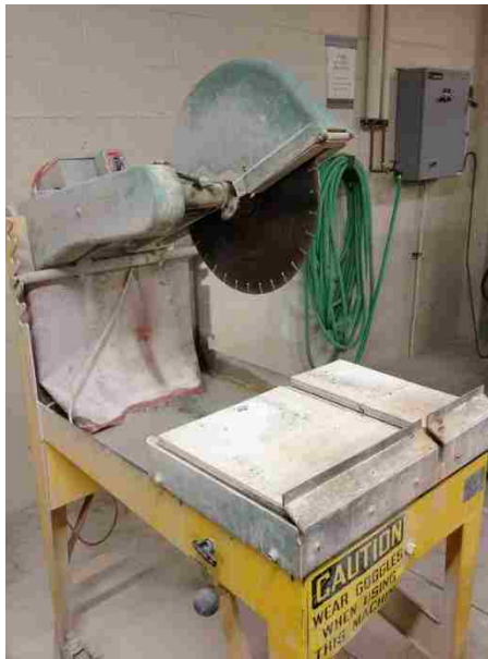
Figure 1 - Wet Saw with Diamond Cutting Blade
