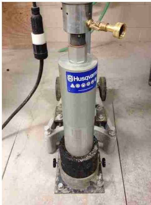
Figure 2 - Specimen Secured in Bottom Jig
