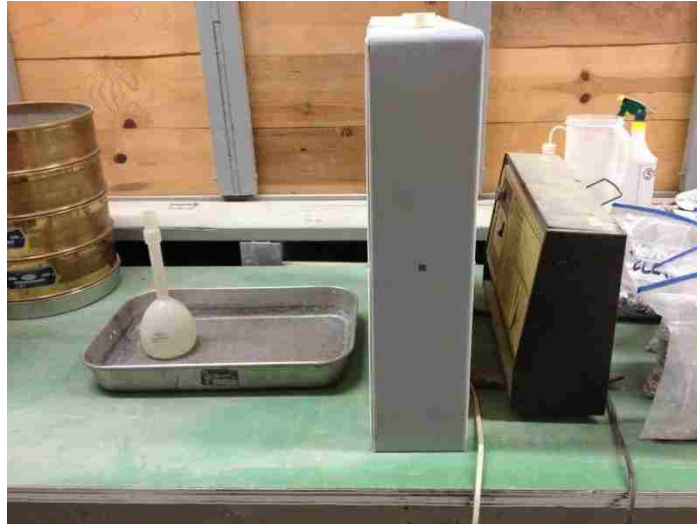
Figure 3.3 - Fine Aggregate Specific Gravity and Absorption Setup
