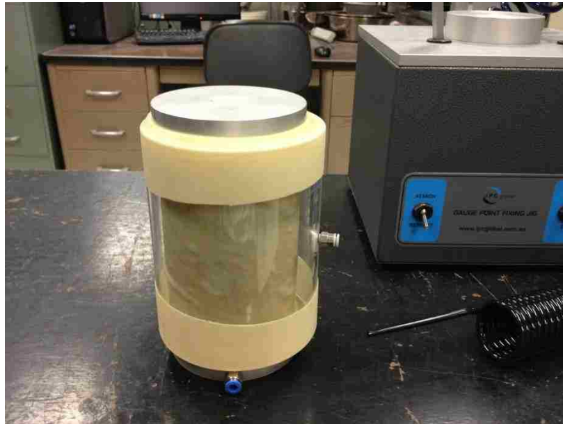
Figure 3.23 - Latex Wrapped Specimen for Flow Number Test
