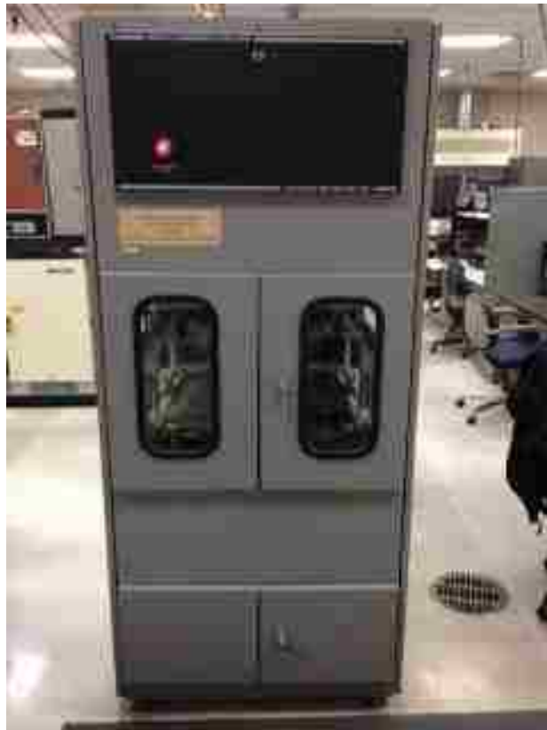
Figure 3.19 - Asphalt Pavement Analyzer (APA)
