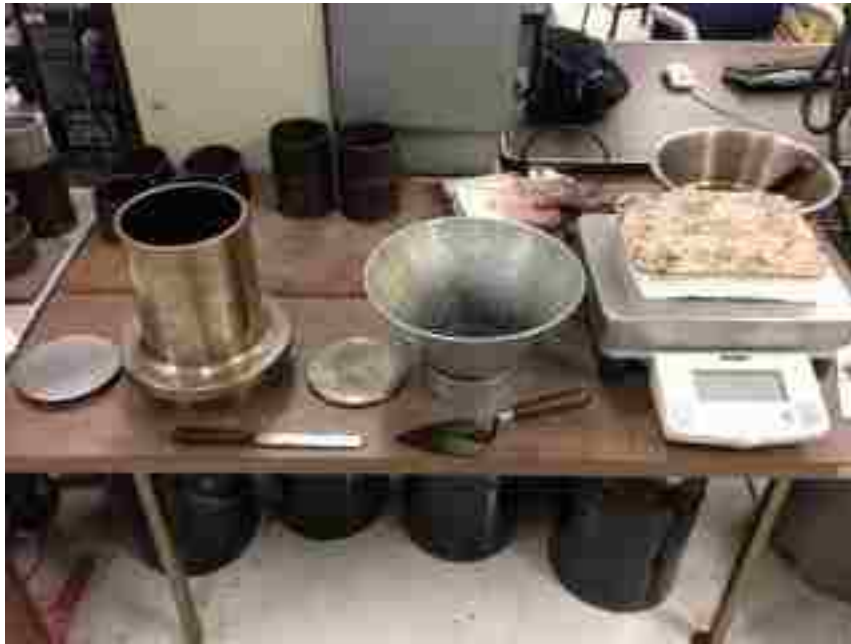
Figure 2 – Mold, Bottom Plate, Top Plate, Funnel, Scale, Assorted Tools
