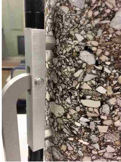
Figure 3.49 – Gauge Points Attached on Specimen Side
