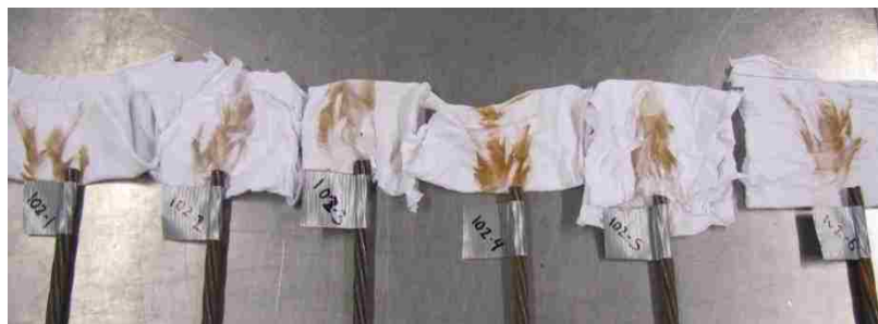
Figure 3.30 – Towel Wipe Results for Strand Type 102
