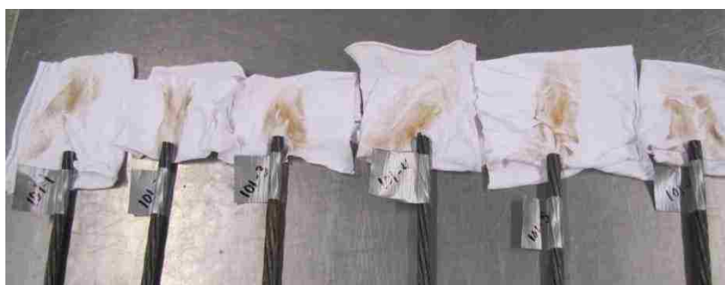
Figure 3.29 – Towel Wipe Results for Strand Type 101
