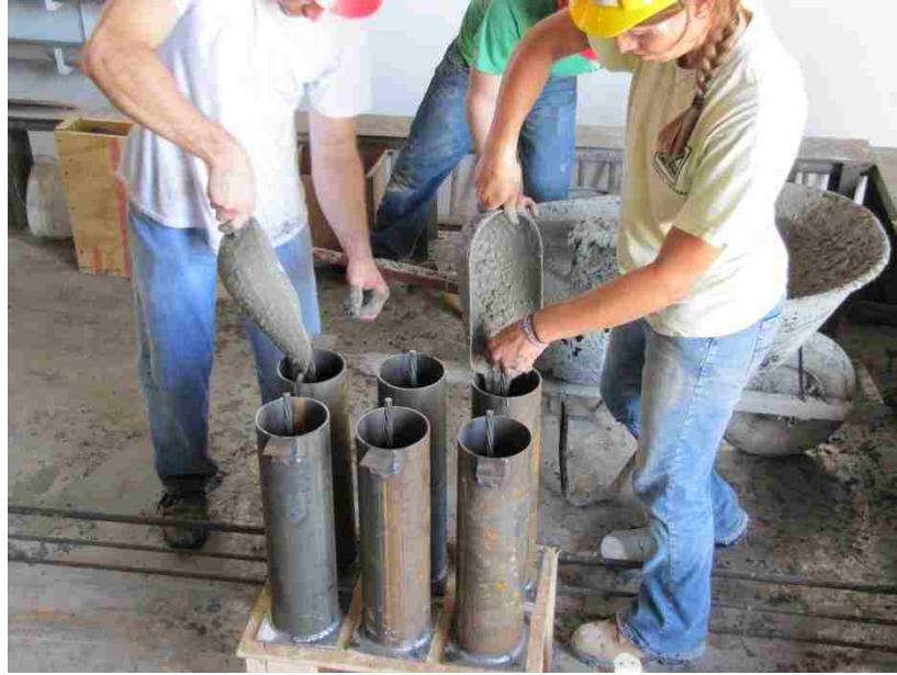
Figure 3.11 – Filling Specimens for NASP Test in Concrete
