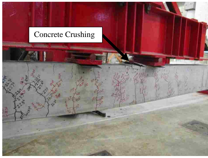
Figure F.31 – S10-2-2_73 at Failure
