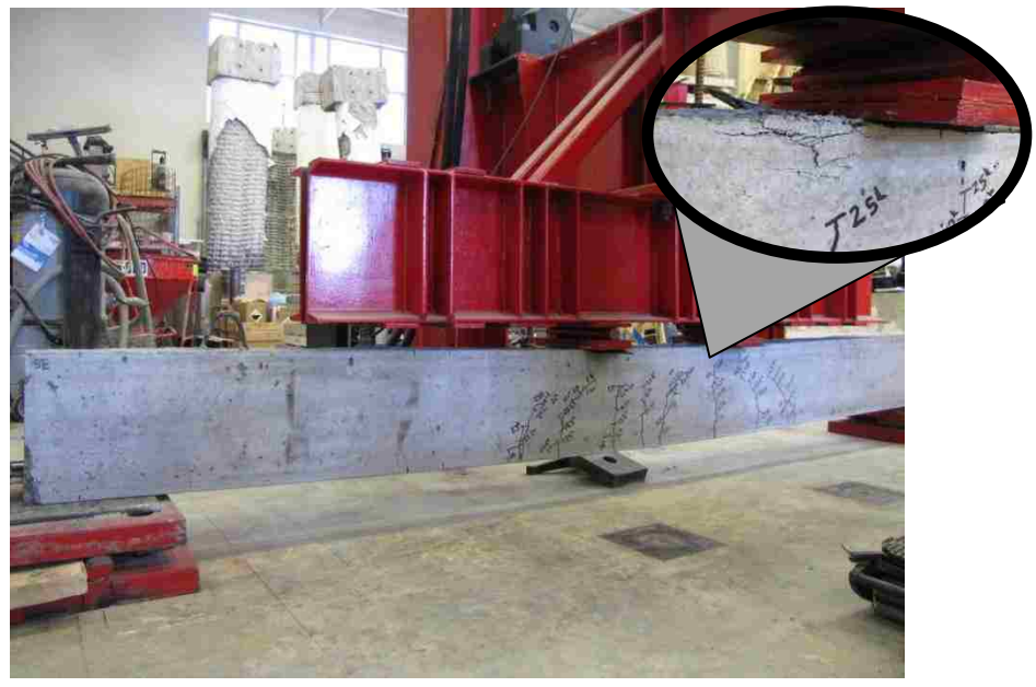
Figure F.1 – C6-2-1_58 at Failure with Detail of Concrete Crushing
