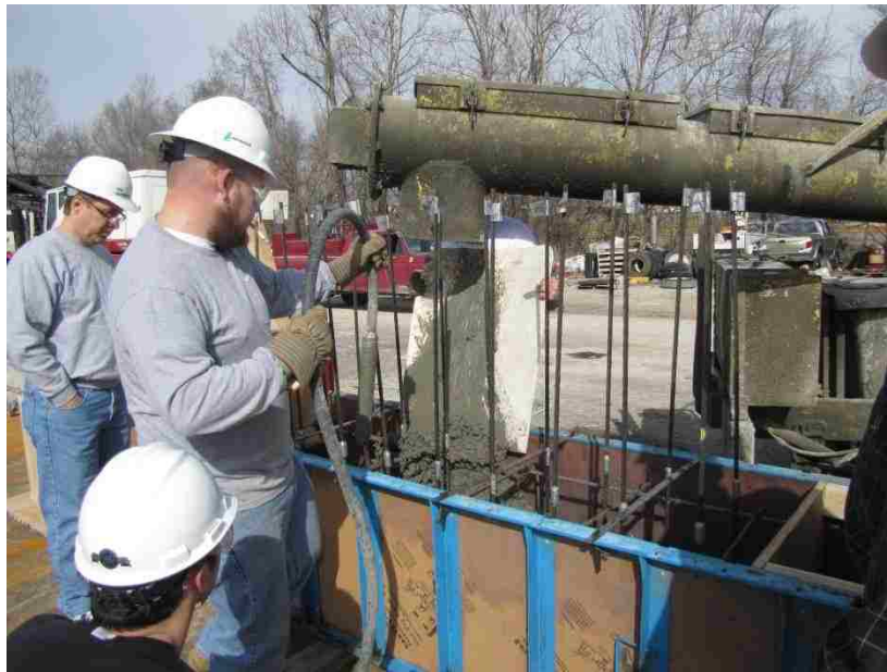
Figure 3.23 – Casting the LBPT Specimen
