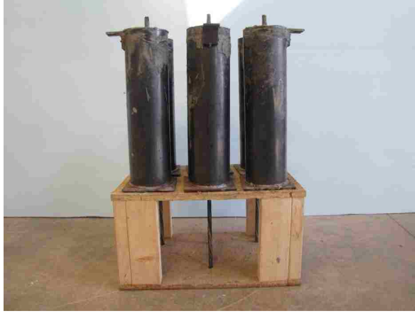
Figure 3.10 – NASP Mold and Strand Setup
