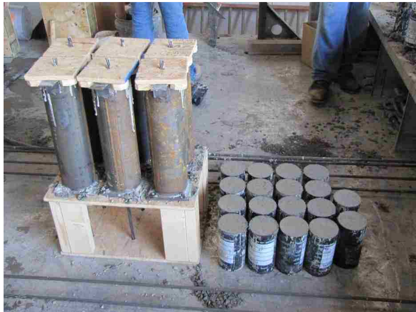
Figure 3.12 – Capped NASP in Concrete Specimens and Cylinders
