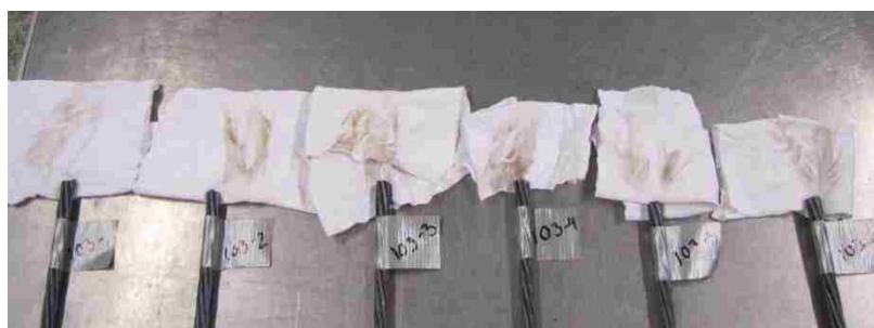
Figure 3.31 – Towel Wipe Results for Strand Type 103
