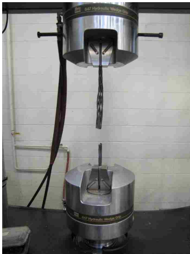
Figure 3.4 – Fractured Tension Test Specimen
