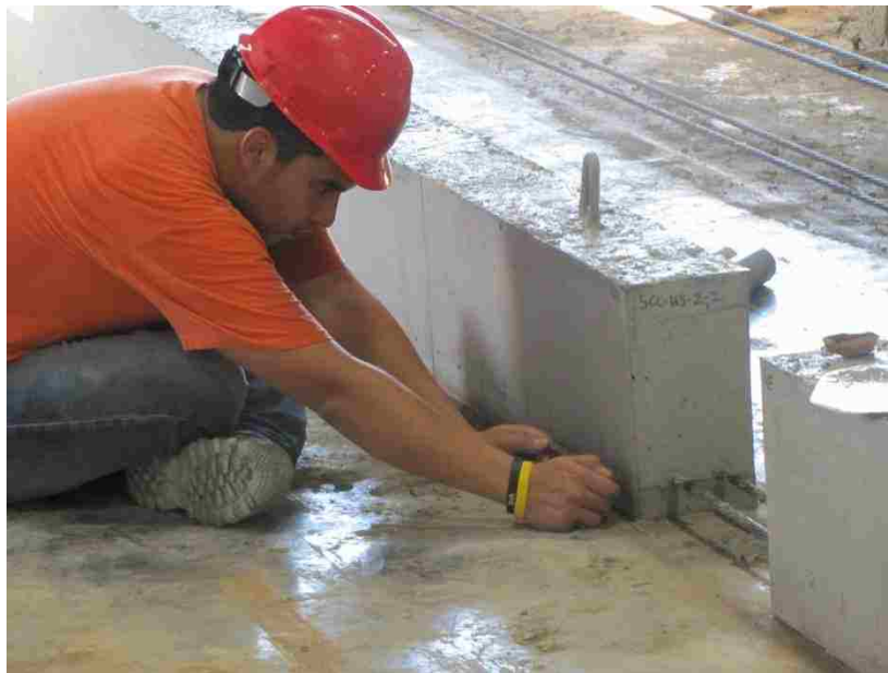
Figure 4.11 – Setting DEMEC Points with Setting Bar
