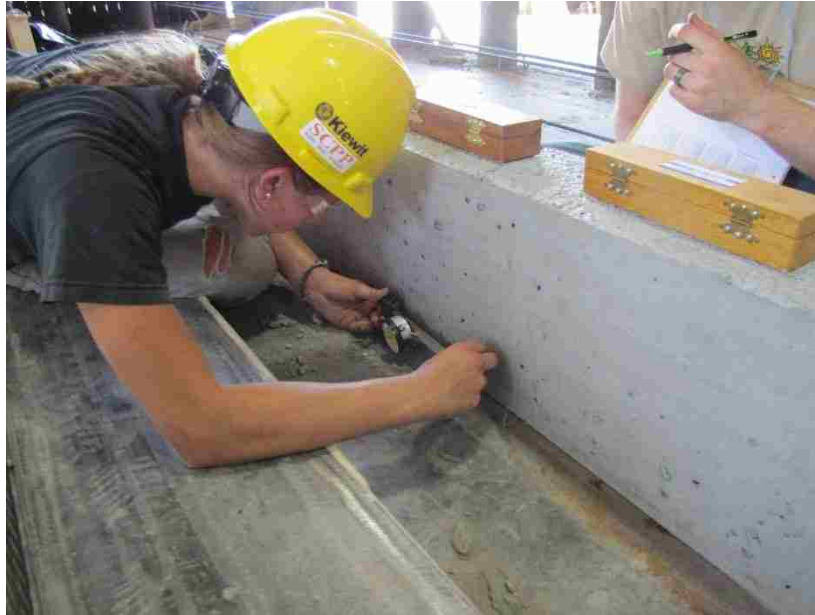
Figure 4.13 – Taking DEMEC Readings
