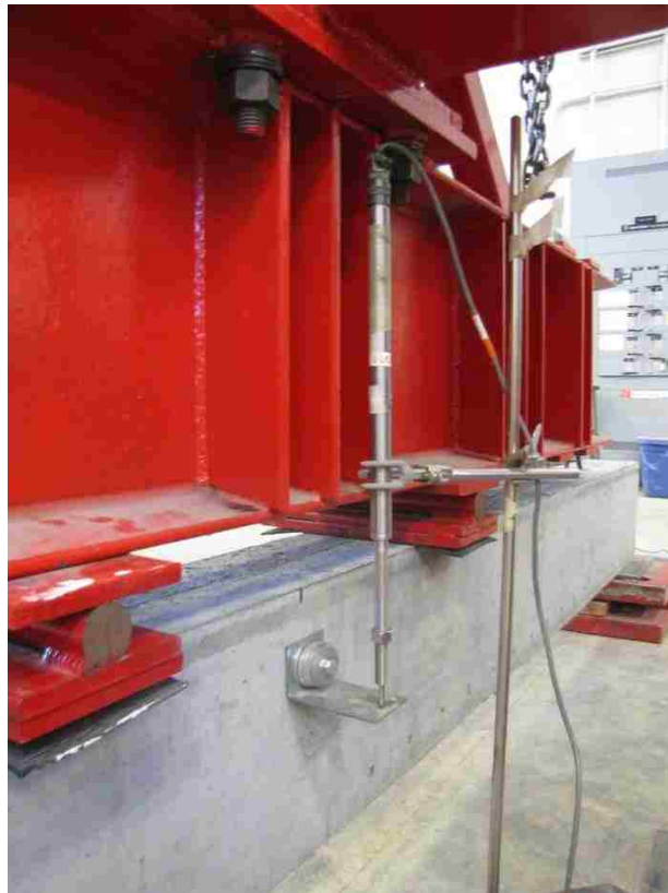
Figure 4.27 – LVDT Setup for Measuring Deflection at Midspan
