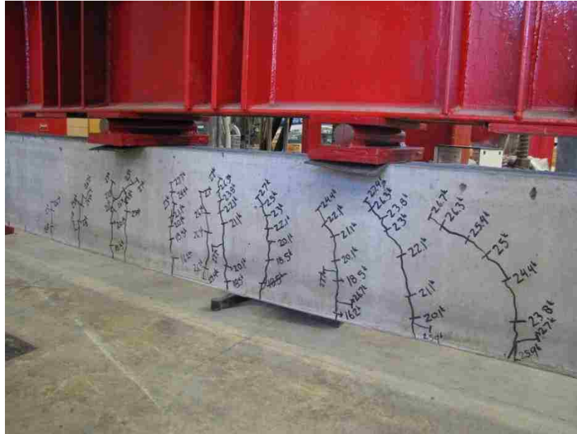
Figure 4.29 – Cracks Marked with Permanent Marker during Development Length Test
