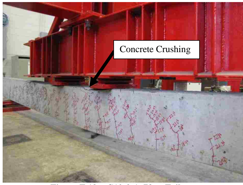
Figure F.19 – C10-2-1_73 at Failure
