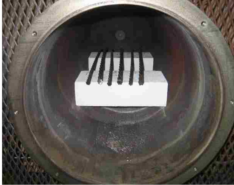
Figure 3.4 Typical heating setup
