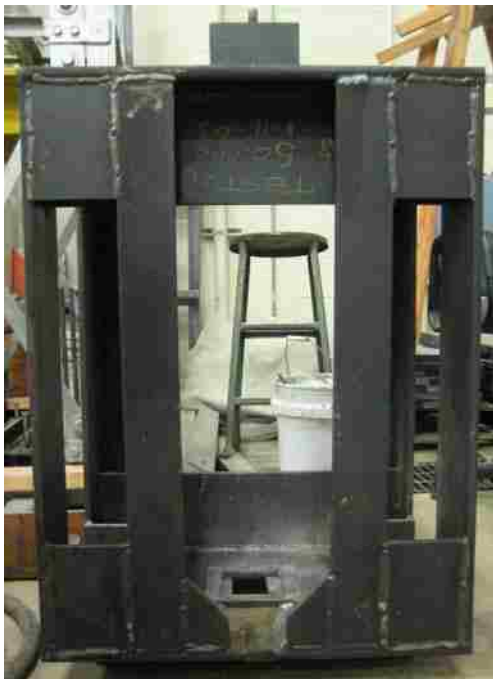
Figure 3.7 Pullout test setup cage prior to testing
