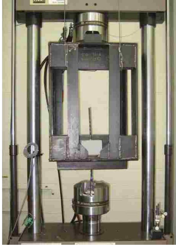
Figure 3.8 Pullout test setup with specimen inside steel cage
