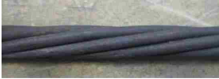
Figure 4.3 Strand exterior after exposure to 1000°F (538°F)
