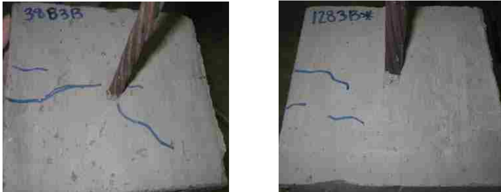
Figure 4.16 Initial hairline cracking noted for each compressive strength (left: 11 ksi, right: 14 ksi)
