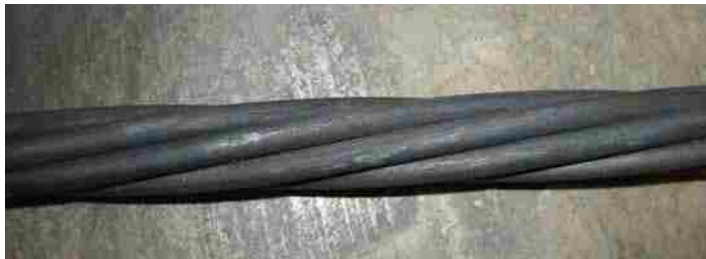
Figure 4.4 Strand exterior after exposure to 1200°F (649°F)
