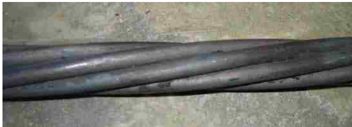
Figure 4.5 Strand exterior after exposure to 1300°F (704°C)
