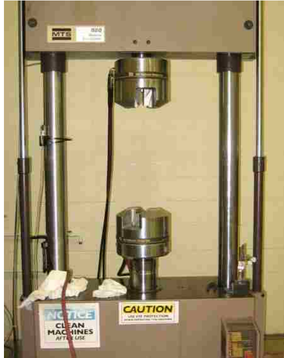
Figure 3.5 MT880 testing machine prior to tension tests
