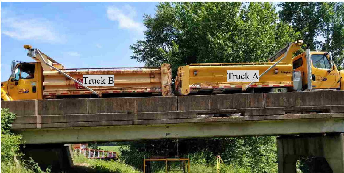
Figure 5.7. Trucks on Span 1 for Load Test
