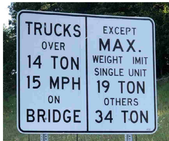
Figure 3.1. Bridge P-0058 Load Posting
