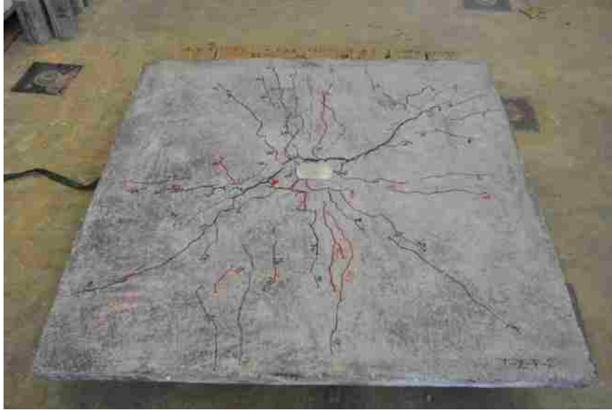
Figure 6.11. Bottom of I-2-6F-2 after testing
