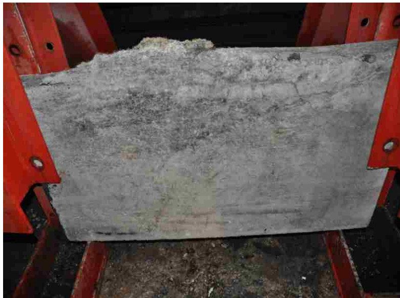
Figure 6.46. Front of H-2-6F-3.5 before detonation
