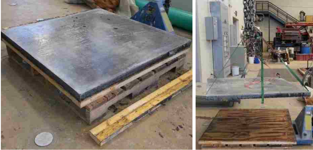
Figure 5.16. Panel de-molding process
