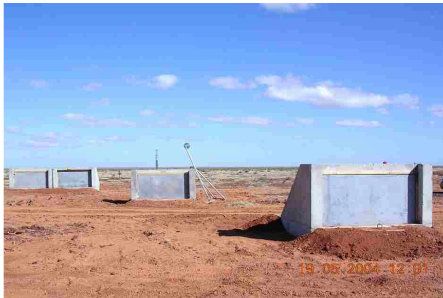
Figure 2.1. "Large-scale blast testing of Ductal protective panels at Woomera in 2004" (Rebentrost, 2006)
