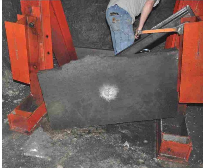
Figure 6.50. Cratering on front face of H-3-6F-3.5 after detonation
