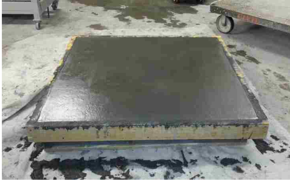
Figure 5.15. Trowel finished panel specimen
