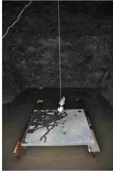
Figure 5.21. Full panel blast test setup
