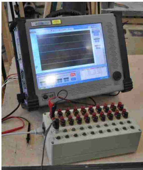
Figure 5.20. Synergy data acquisition system
