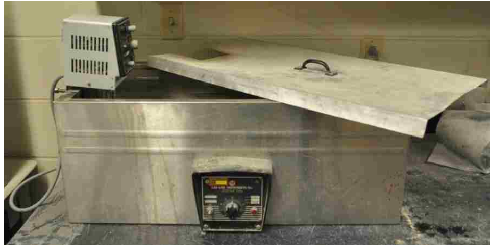
Figure 4.24. Heat curing tank used for small scale curing
