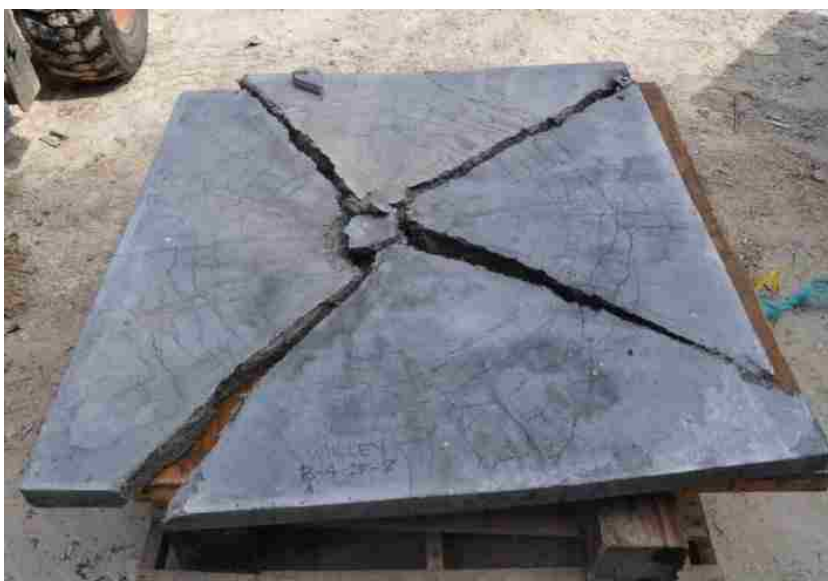
Figure 6.16. Panel B-4-2F-2 damage after detonation
