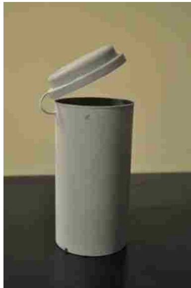
Figure 5.6. Splitting tensile specimen mold
