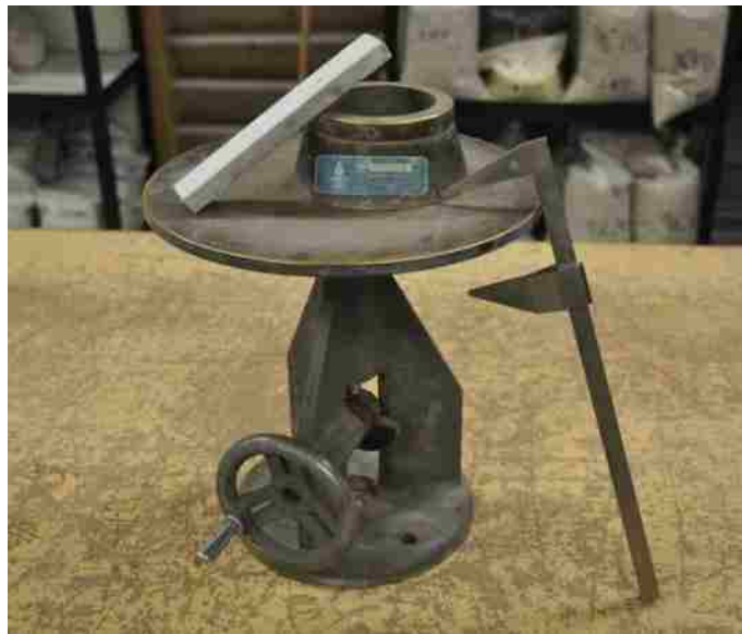
Figure 4.26. Flow testing equipment
