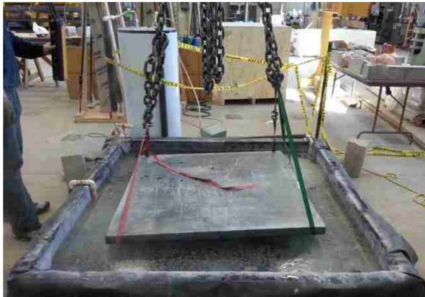
Figure 5.17. Panel being added to heated curing bath
