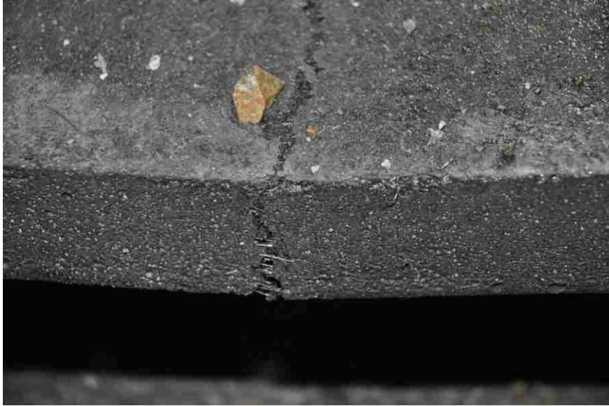
Figure 6.33. Crack development after detonation
