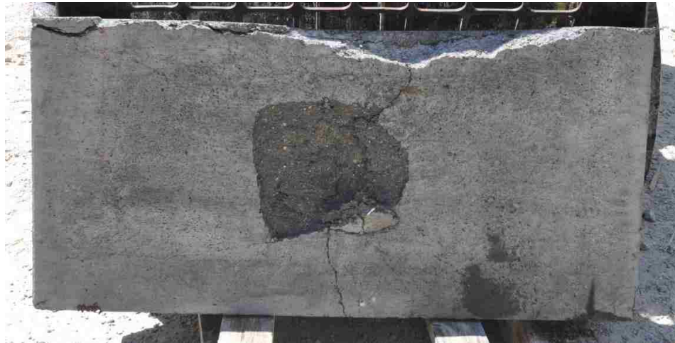
Figure 6.61. Tension face of panel H-7-6F-3.5 after detonation
