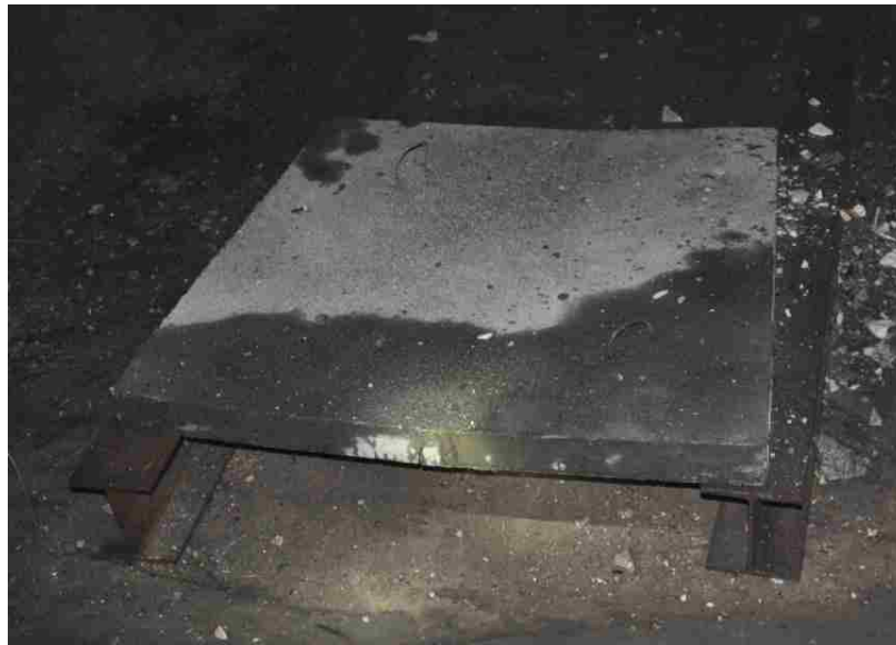
Figure 6.27. Top face of B-1-6F-3.5 after second detonation
