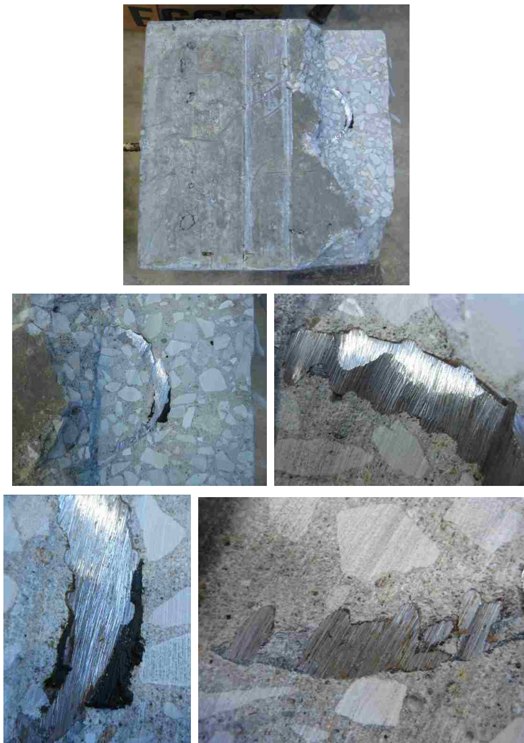
Figure C.2. Dissected specimen BE-5-180-0
