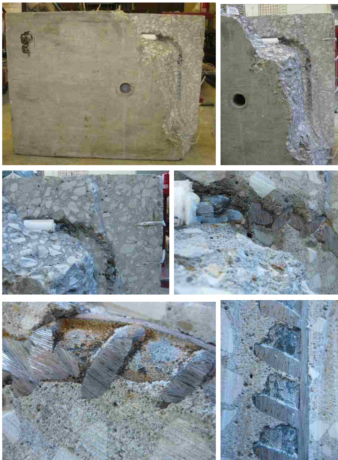
Figure C.5. Dissected specimen BE-8-90-90
