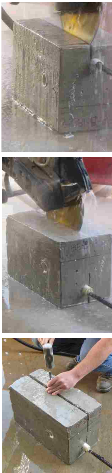
Figure C.1. Dissection process (specimen BE-5-180-90 shown)
