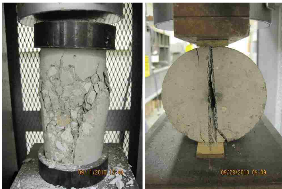
Figure A.1. Compression and splitting tensile strength tests
