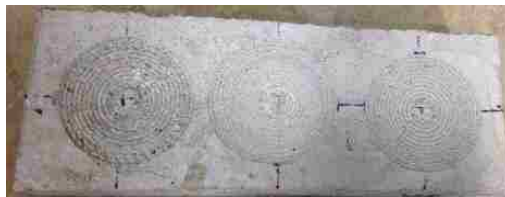
Figure 3.25: 35% 28d Abrasion Specimen post test
