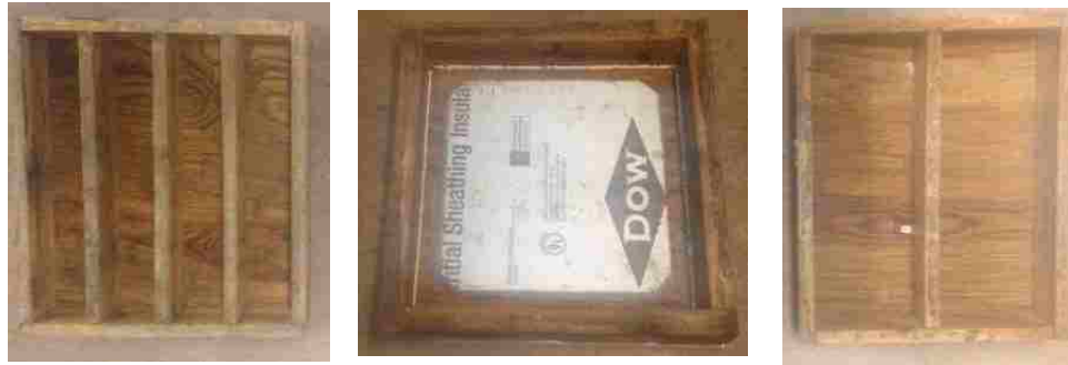
Figure 3.8: Formwork for Durability Specimens.
