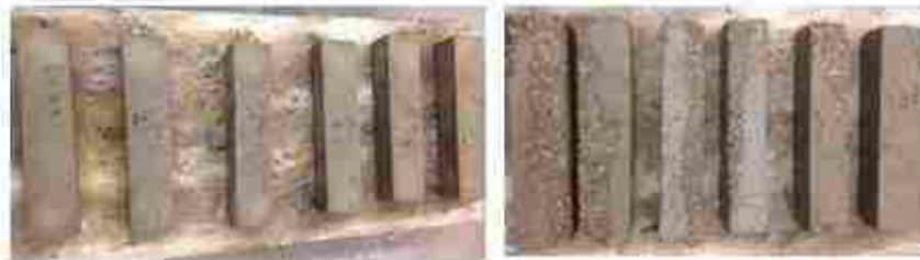
Figure 3.27: 60T Freeze-Thaw Specimens (Left: Before, Right: After)
