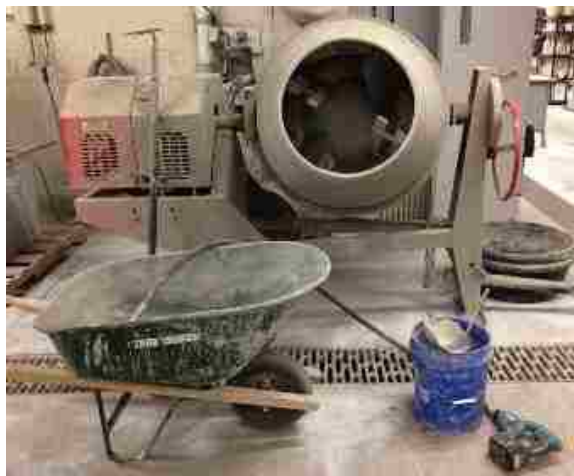
Figure 3.1: 6cft Concrete Mixer (0.222 yd 3 )
