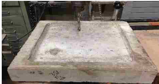
Figure 3.26: 35% 90d Chloride Ion Penetration Specimen
