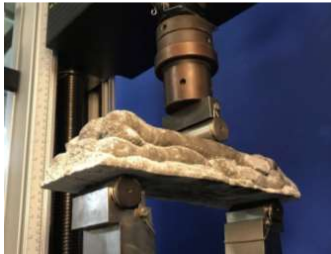
Figure 3.24. Manual Printed Beam Three-Point Bending Setup
