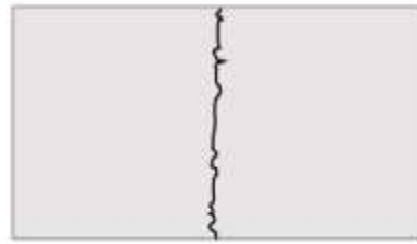
(a) Vertical Crack in Cast Beam
