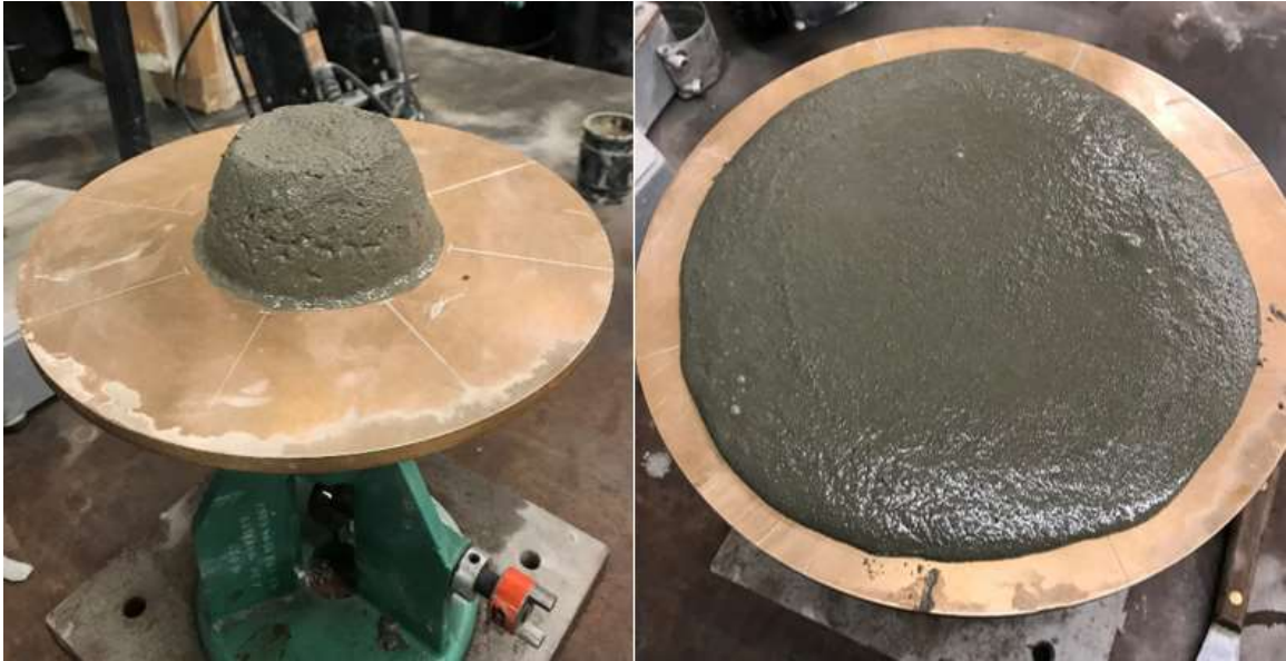
Figure 3.10. Flow Table Test Before and After 25 Table Hits
