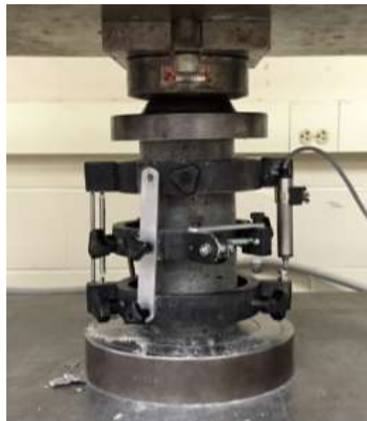
Figure 3.4. Modulus of Elasticity Test Set Up
