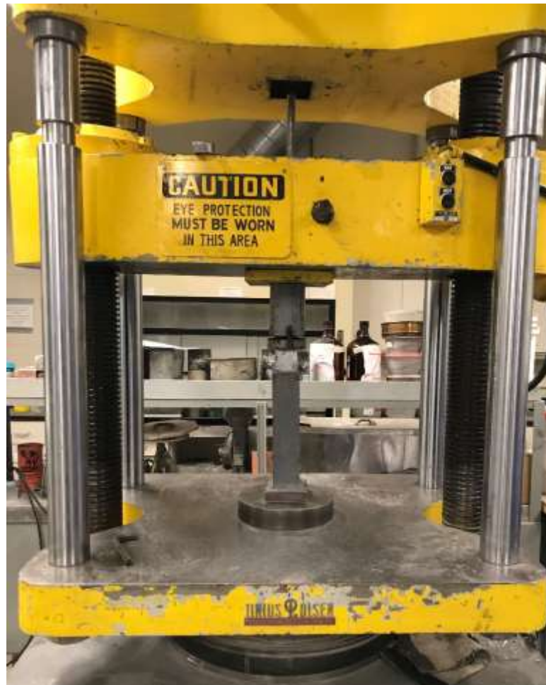
Figure 3.22. Cube Compression Test Setup
