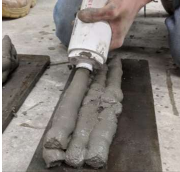
Figure 3.20. Beam Manual Printing Process
