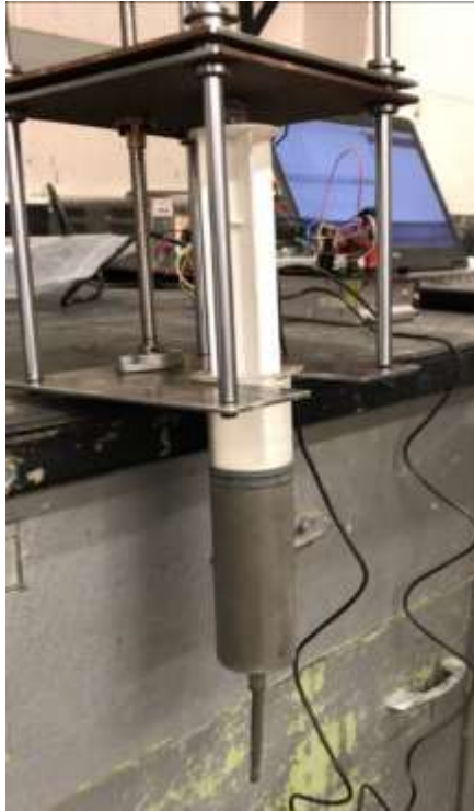
Figure 3.19. Extrusion Test in Progress
