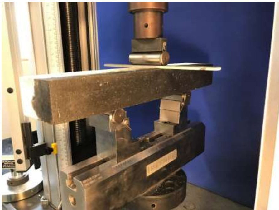
Figure 3.23. Cast Beam Three-Point Bending Setup
