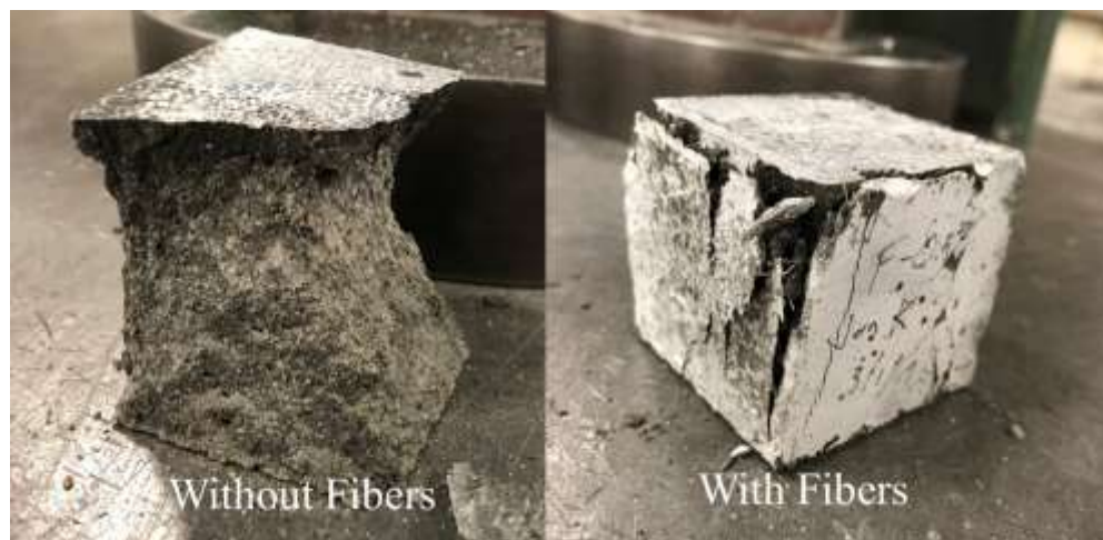
Figure 4.35. Cube Compressive Failure Comparison
