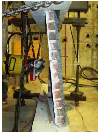
(c) Wall Failure
