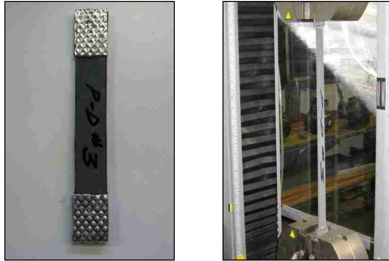
Figure 3.3. Testing of Polyurea Coupon
