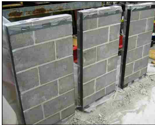
Figure 6.2. Phase 2 URM Walls Prior to Strengthening
