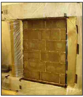
(a) Primed URM Wall
