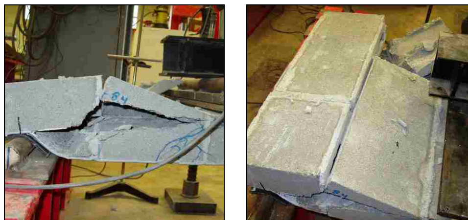
(a) Separation from Polyurea
