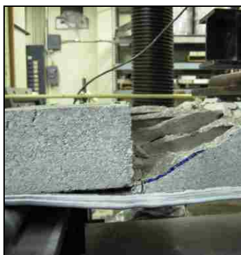
(c) Flexural-Shear Failure
