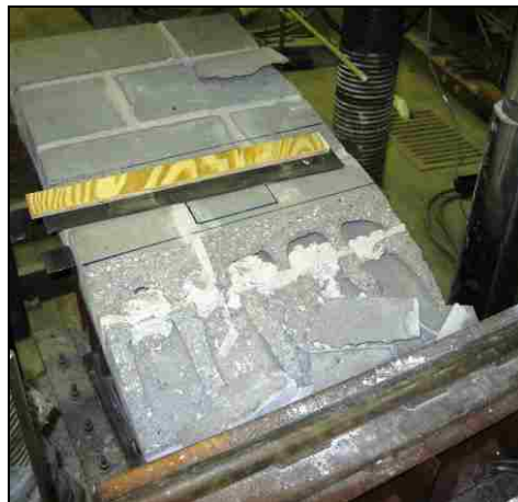
(c) Fracturing of Masonry
