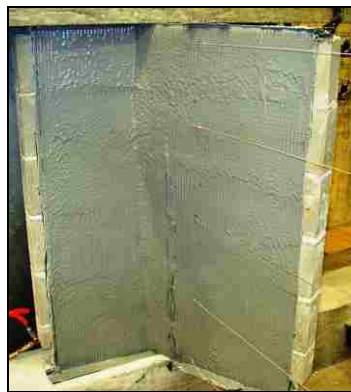
(a) Bending About Vertical Axis
