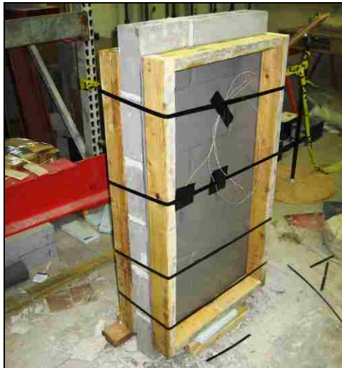
Figure 6.6. Braced URM Wall
