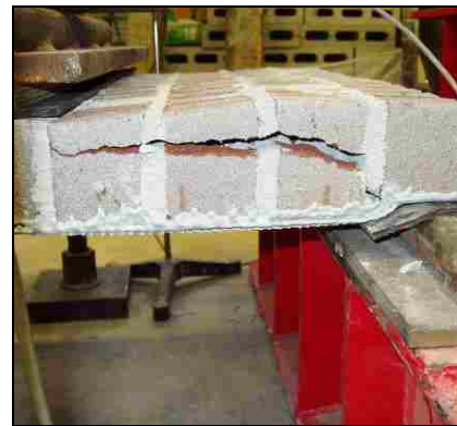
(b) Flexural-Shear Cracking
