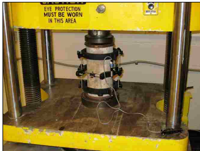
Figure 3.11. WF-FA Compression Testing
