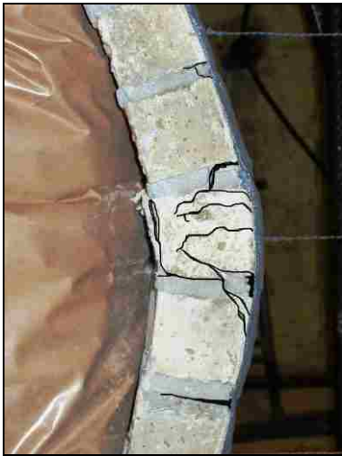
(b) Flexural Cracks in WF-FA
