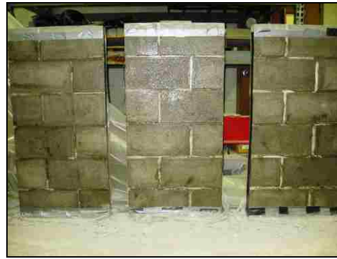
(b) Primed URM Walls
