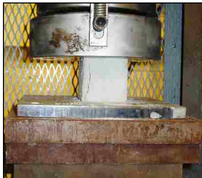
Figure 3.6. Mortar Cube Testing
