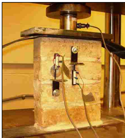
Figure 3.13. Compression Testing of WF-FA Prism
