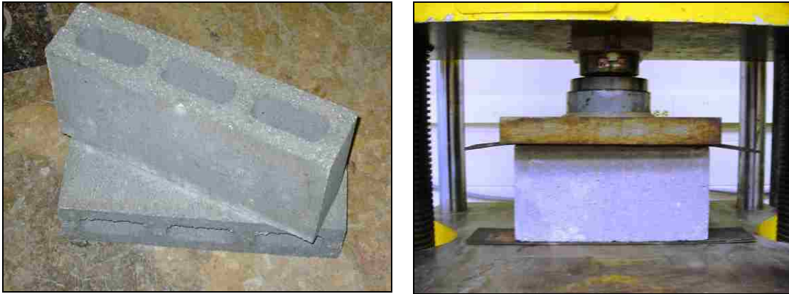
Figure 3.8. Testing of Individual Concrete Masonry Units
