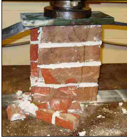
Figure 3.12. Compression Testing of Clay Prism
