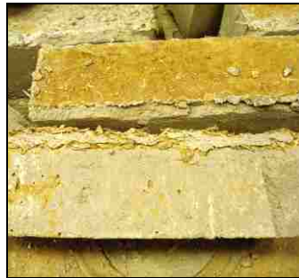
(c) Crushing of WF-FA Brick Units
