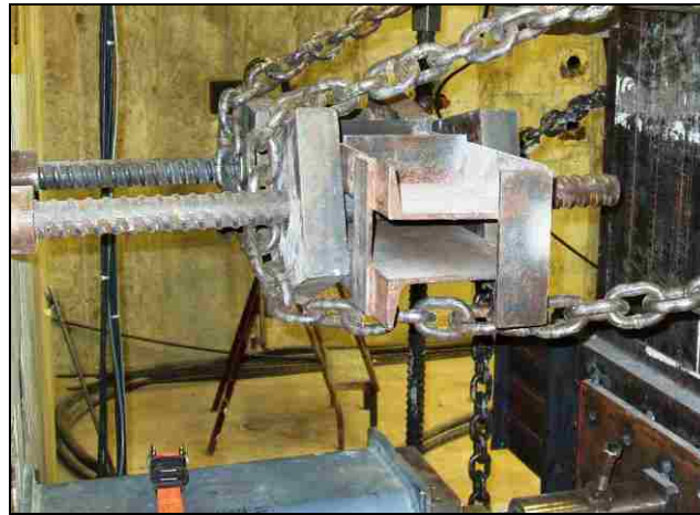
Figure 5.9. Chain Restraint System
