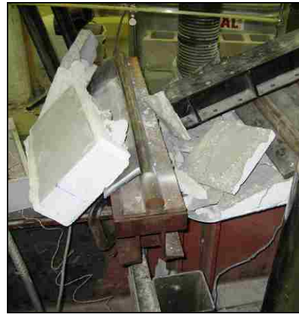
(b) Debonding of Masonry
