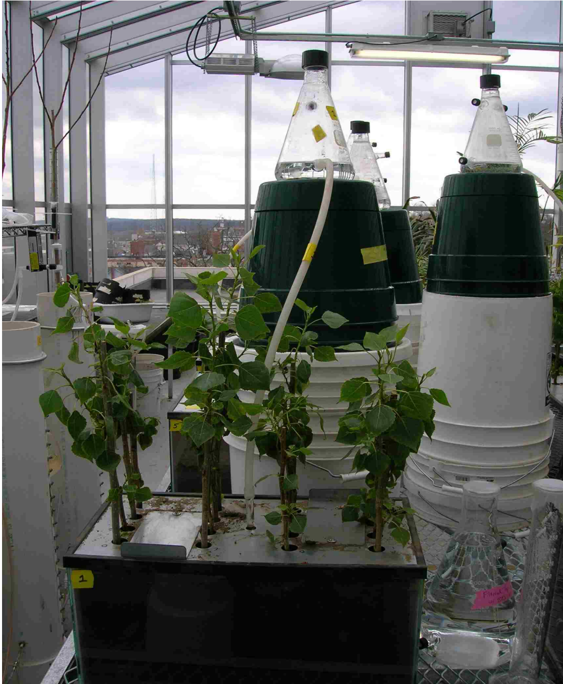
Figure 3.2 Picture of Reactor 1 after construction and planting were complete. Note the one liter Erlenmeyer flask attached to the centered glass feed tube by Teflon lined tubing for water addition.
