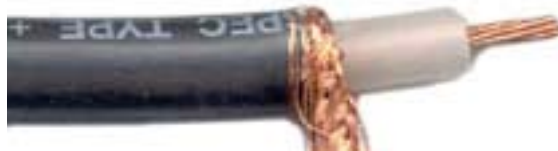
Figure 5.1 Picture of the Coaxial Cable Tested (Cerri et al., 2005)
