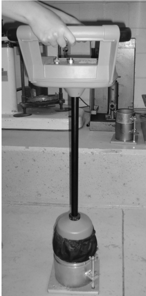
Fig. 2 – BCD testing on a compacted soil sample in a 6” split mold.
