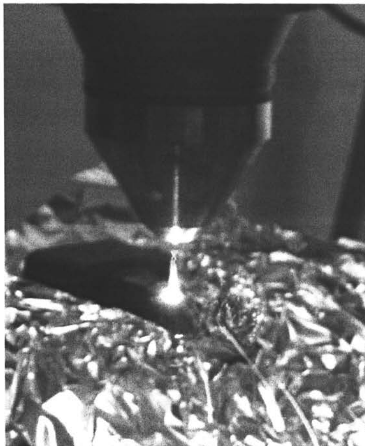
Figure 3.2 LAMP Deposition Process using the Laser Beam
