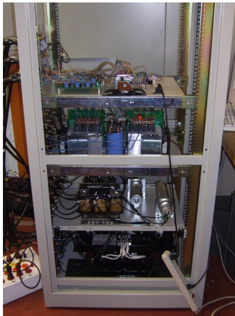
Figure 5.4: Internals of the FACTS device.
