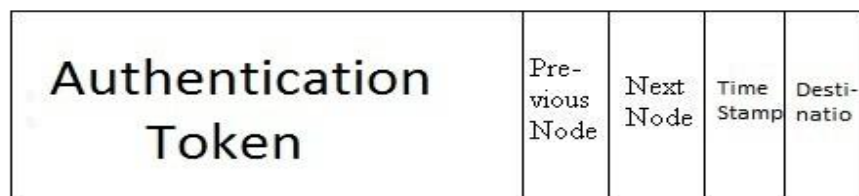
Figure 4.5 Receipt structure stored at each intermediate node and destination
