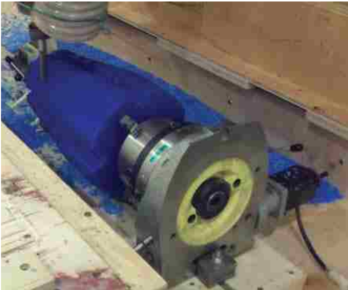
Figure 9: Part and resulting waste after CNC routing
