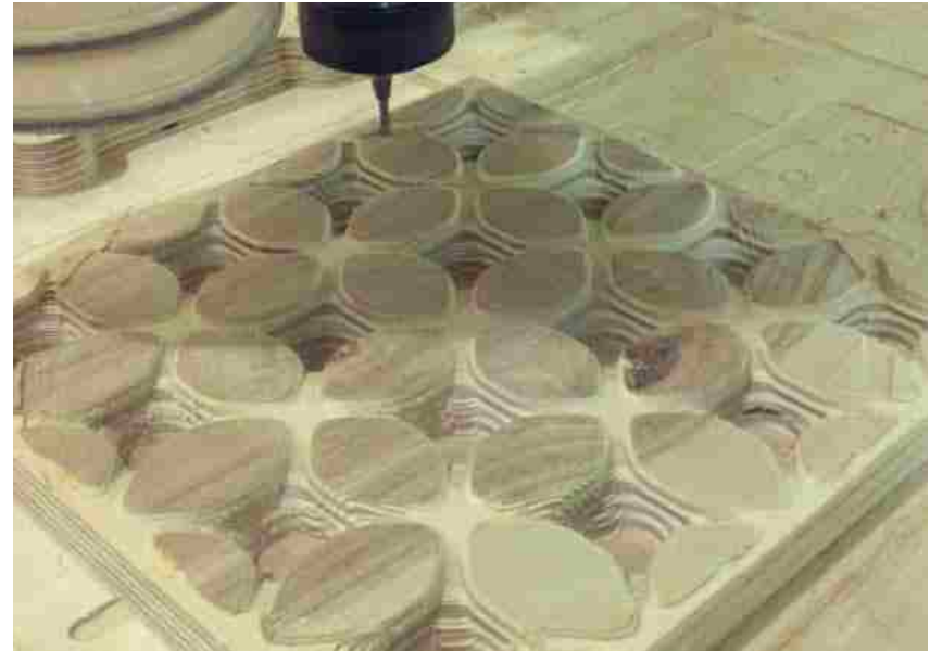
Figure 33: CNC routed plywood mold for second [m]form prototype membrane
