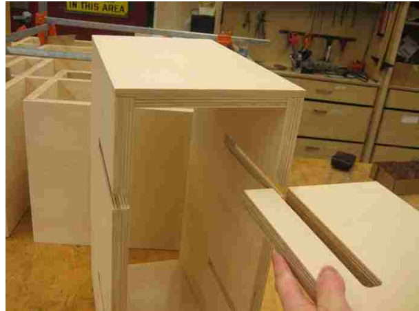
Fig. 9.5 Interlocking slot detail and assembly
