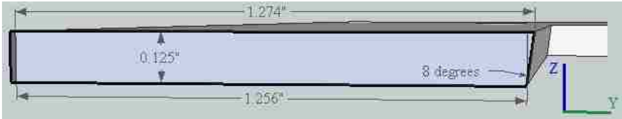
Figure E-71. Cross sectional view of the 20x20 cm 2 upper trimmer aluminum plate in the in-plane dimension illustrating the thickness and lateral dimensions of the plate.
