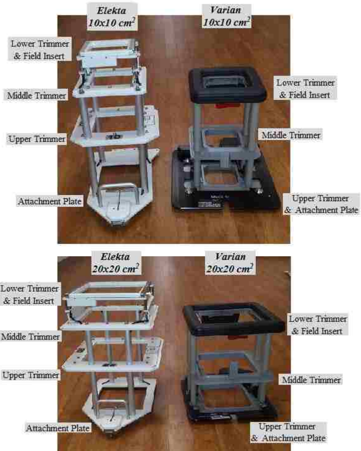
Figure 1-8. Comparison of the current clinical Elekta and Varian applicator designs for the 10x10 and 20x20 cm 2 sizes. The locations of the field insert, the upper, middle and lower trimmers, and the attachment plate are labelled for each applicator.
