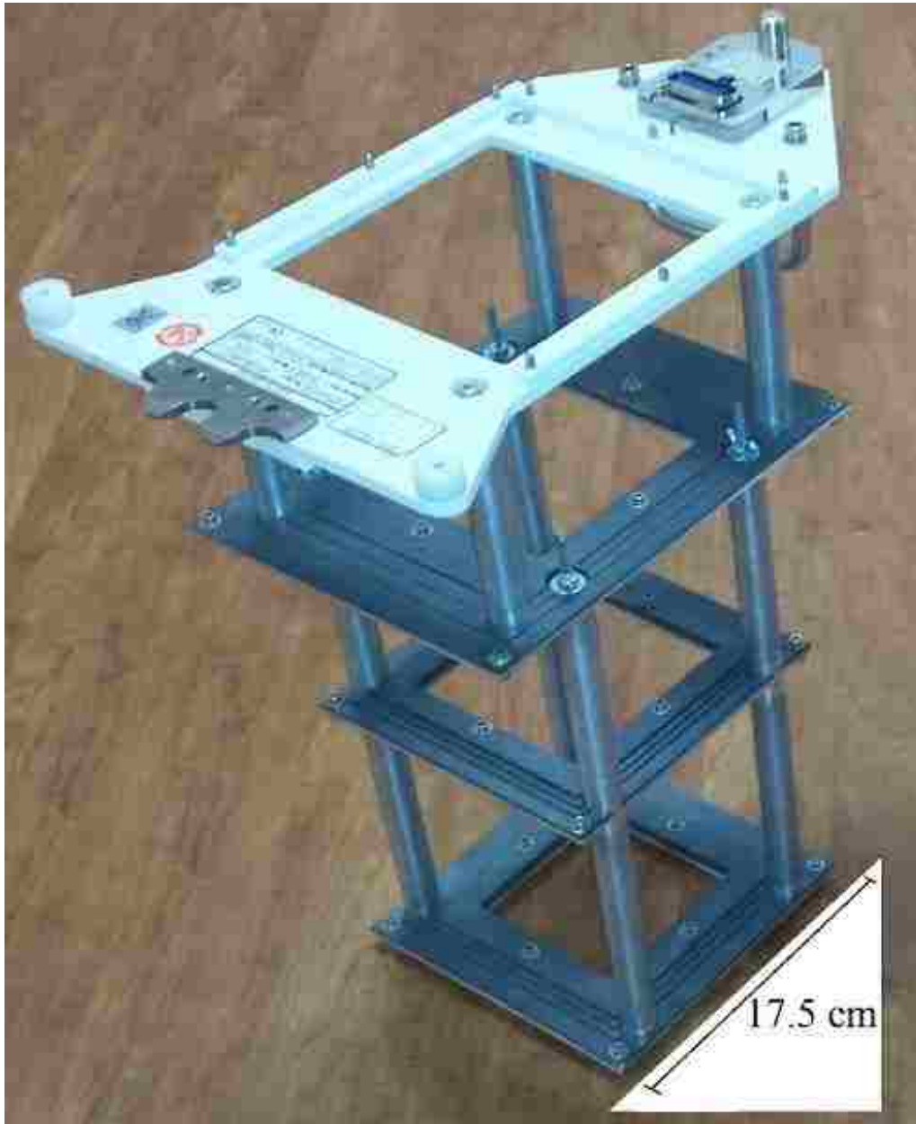
Figure 7-2. Fabricated 10x10 cm 2 applicator prototype.
