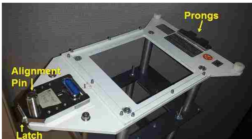
Figure 1-10. Attachment plate of the Elekta Infinity accelerator with the prongs, alignment pin, and latch labelled.
