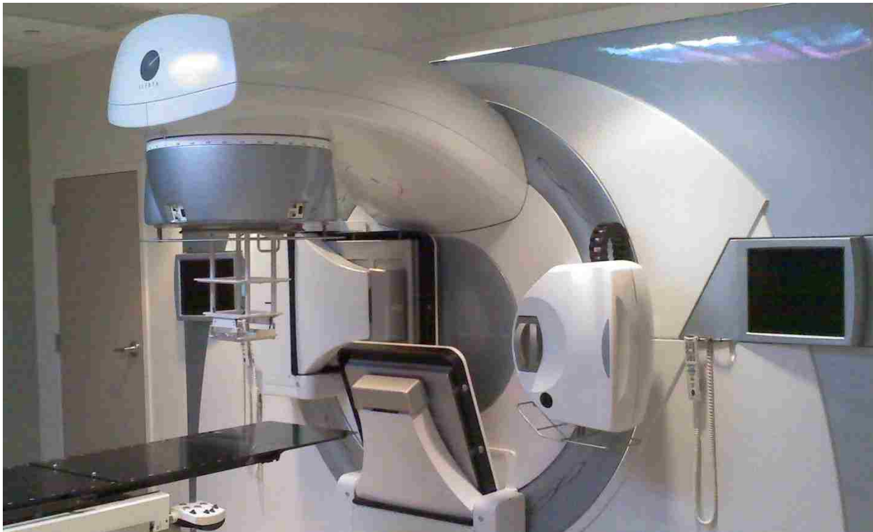
Figure 1-5. Elekta Infinity accelerator with the 14x14 cm 2 applicator attached to the treatment head (from Harris, 2012).
