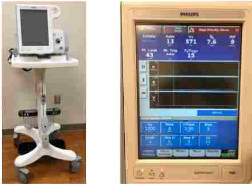
Figure 2.1. Left: Philips Respironics V60 BIPAP ventilator. Right: Philips BIPAP LCD touchscreen which displays monitored patient parameters such as the tidal volume and breathing period as well as the real-time pressure, flow, and volume waveforms.
