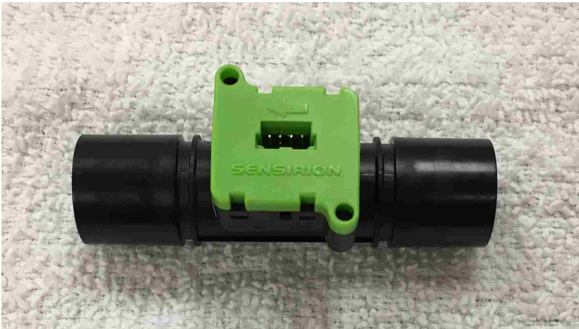
Figure 2.9. Sensirion SFM 3000 mass flow meter.
