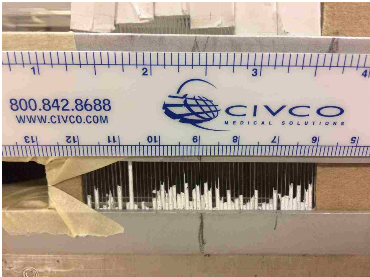
Figure 25. Example of an image used for final fiber location indexing showing the fiber ribbon at the exit face of the magnet block.
