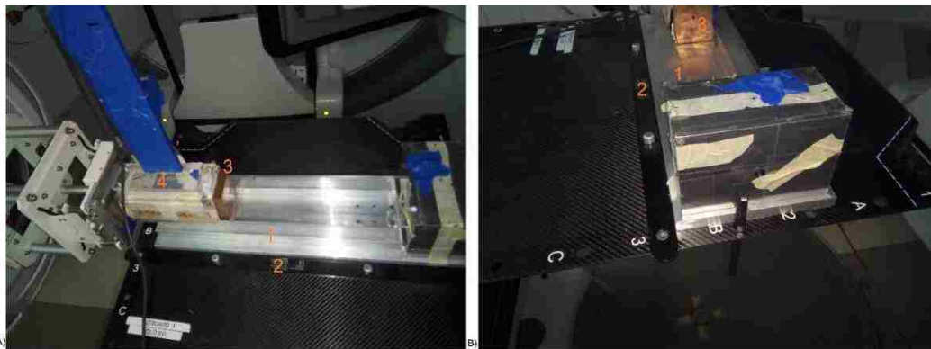
Figure 44. Spectrometer setup and placement on patient treatment couch. 1 is a metal baseplate; 2 is the accessory mounting bar attached to the couch; 3 is a copper plate mounted to the baseplate; 4 is the spectrometer. A) shows the overall placement on the couch. B) Reproducible setup was achieved in the beam-axis direction by moving the baseplate back to make contact with a pen placed in one of the couch mounting holes.
