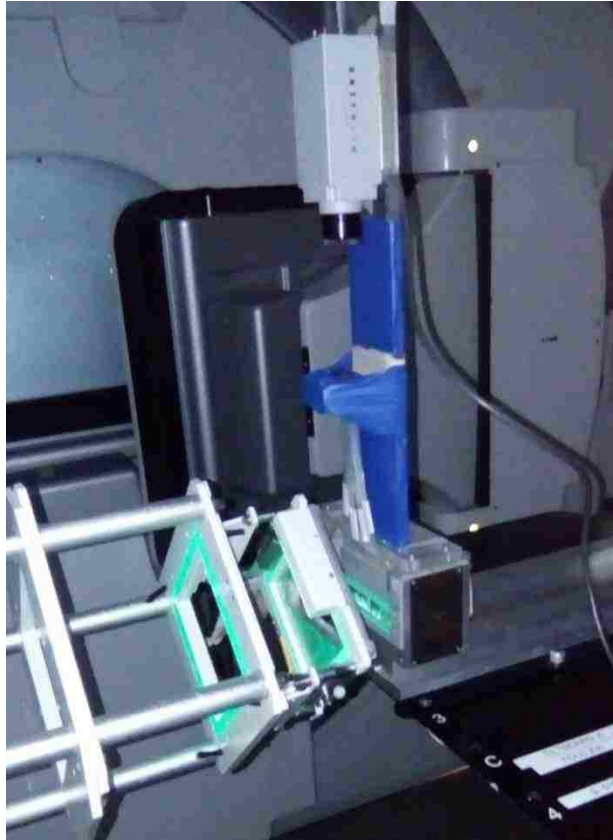
Figure 41. Setup for flood shot acquisition setup. The spectrometer is rotated 90° from its normal orientation.
