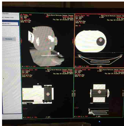
Figure 2.12: Three orthogonal views of a single phase of 4D CT reconstruction and a 3D rendering of the phantom (top left).
