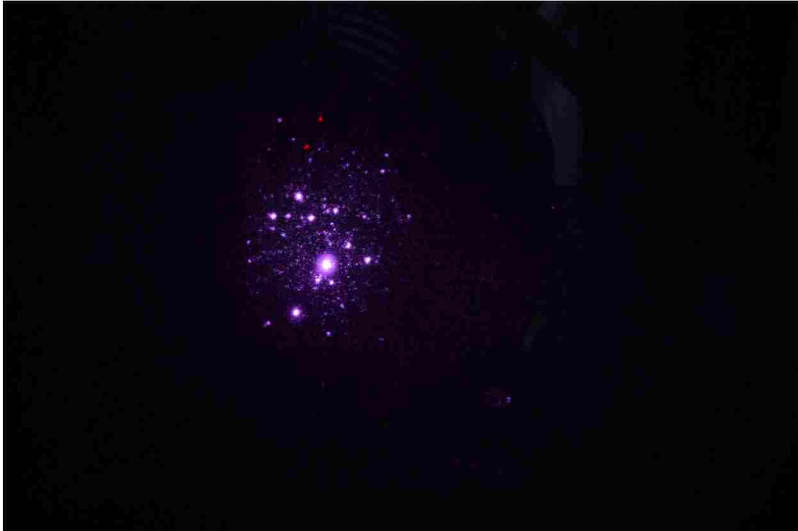
Figure 4.3: Example of long-exposure photograph of the interferometric-beam scatter from the surface of a test mass.
