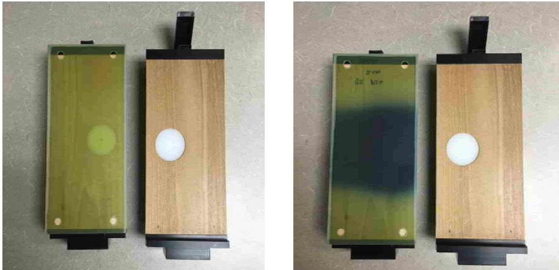
Figure 17: Radiochromic film piece cut flush with cedar film and tumor insert with punched registration holes before delivery (left) and after delivery (right).
