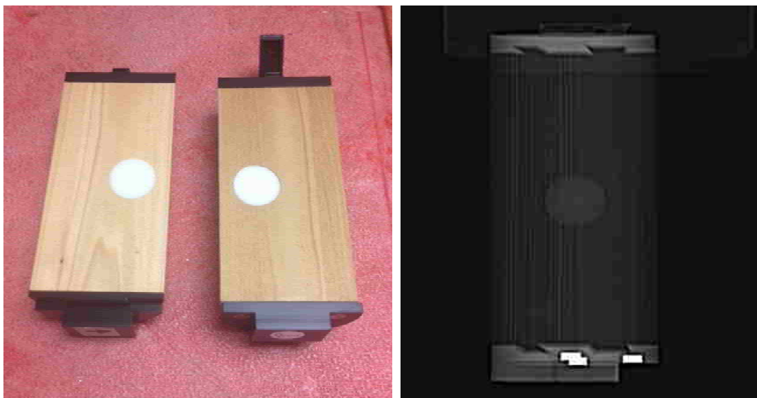
Figure 7: Cedar lung tumor insert (left) and CT scan of cedar lung tumor insert (right).
