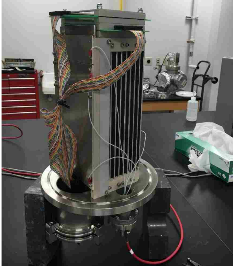
Figure 6-3: The ion chamber electronics being wired in the lab at LSU for testing.
