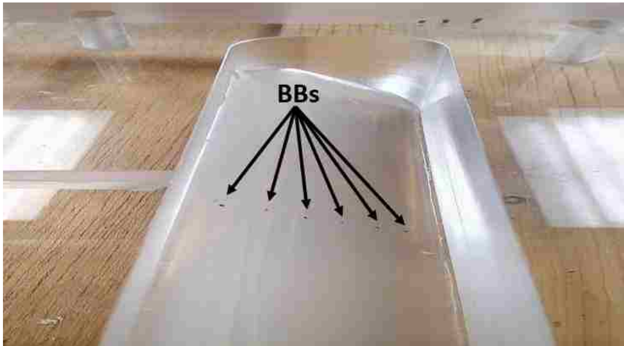
Figure 4.16: View looking down on sample holder plate, showing BBs in place on the slanted surface of the gel slab.
