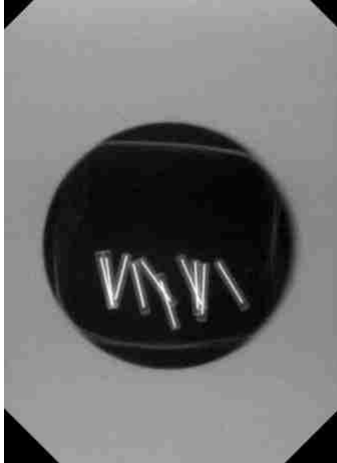
Figure 4.2: Representative projection image acquired with the XDR sensor of 10 LDRBT seeds (titanium shell is \approx 5 mm long with diameter \approx 0.8 mm, silver core is \approx 3.5 mm long with diameter \approx 0.3 mm) implanted in a Styrofoam plug.
