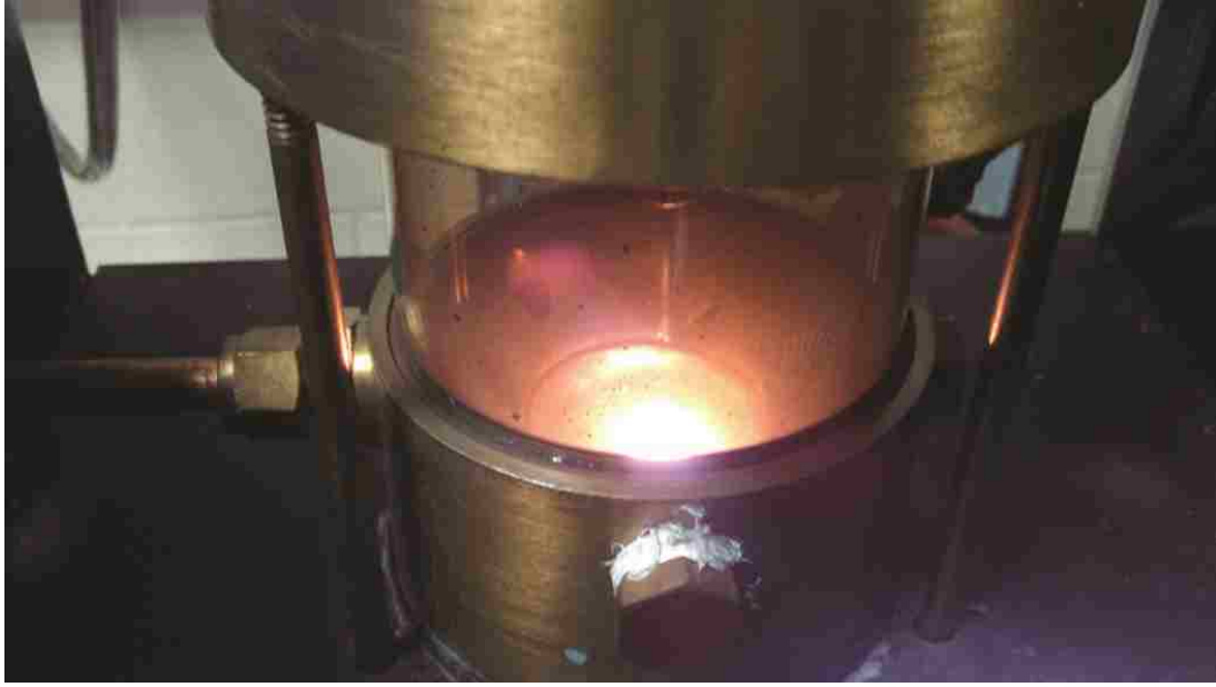
FIGURE 3.4: Synthesis of polycrystalline \text{Fe}_{1-x}\text{Co}_x\text{Si} samples in an arc furnace.
