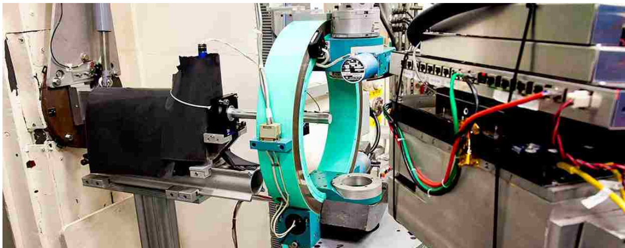
Figure 2-6 Four-Circle diffractometer for HB-3A at Oak Ridge National Lab. Picture adapted from website: https://neutrons.ornl.gov/hb3a .
