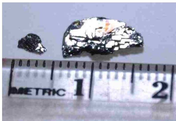
Figure 2-2 BaMn 2 Sb 2 crystals grown by the Sn flux method. Natural layered structure can be observed.
