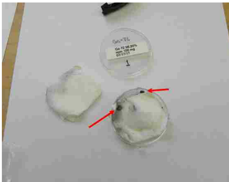
Figure 2.9. The damaged ^{72}\text{Ge} sample received at LANL. Two distinct layers can be seen here and a few others are amongst the padding.
