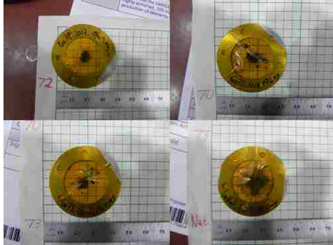
Figure 2.10. The reassembled germanium samples. Some turned out better than others. The least important sample, ^{Nat}\text{Ge} (lower right), was assembled first and the most important, ^{72}\text{Ge} (upper left), was assembled last. This choice paid off as the most important sample wound up being the most intact.
