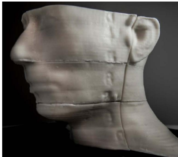
Figure 1.3. A 3D printed head phantom designed from imaging data. This phantom was adapted in post-processing to be able to utilize multiple forms of dosimeters, and printed with ABS plastic using fused deposition modeling. Image adapted from Ehler et al., (2010).
