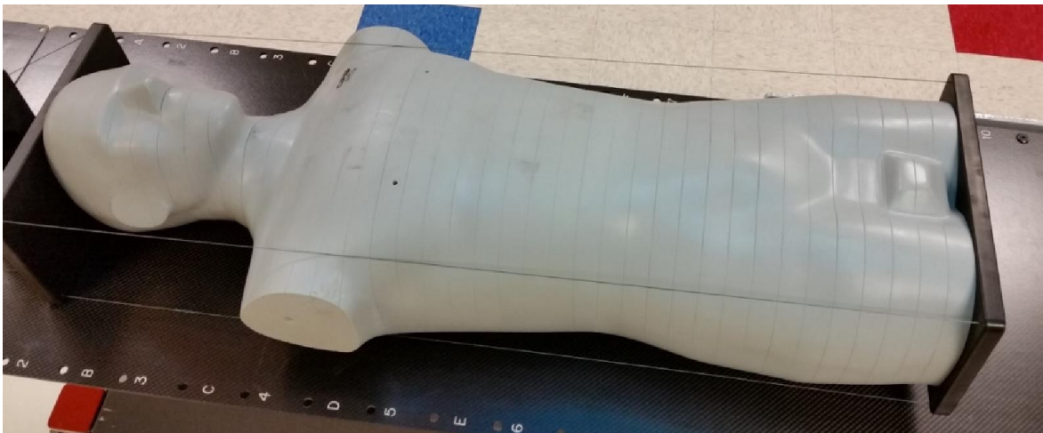
Figure 1.2. An anthropomorphic adult male phantom designed from reference anatomy. This phantom was constructed from multiple tissue equivalent epoxy resins and fabricated using molds. The design is compatible multiple types of dosimeters.
