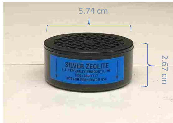
Figure 1.3. Photograph of AgZ cartridge from F & J Specialty Products, INC. used in this project. Arrows
