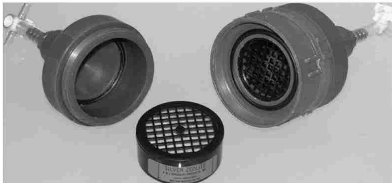
Figure 1.4. Photograph of an AgZ cartridge between two holders for a CAM. (Wang and Matthews, 2006).
