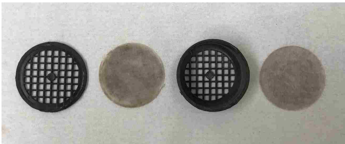
Figure 2.1. Components of an AgZ cartridge. From left to right: lid, filter paper, canister, and second filter paper.
