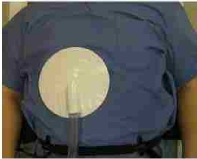
Figure 2.1: The hepatic driver (Resoundant, Inc. Rochester, MN) provided with the MRI system.
