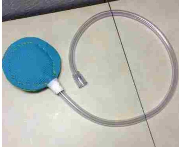
Figure 2.2: The ergonomic flexible driver designed for MRE brain scans. The flexible reducer was connected the passive driver's tube to the active driver located outside the scanner room.
