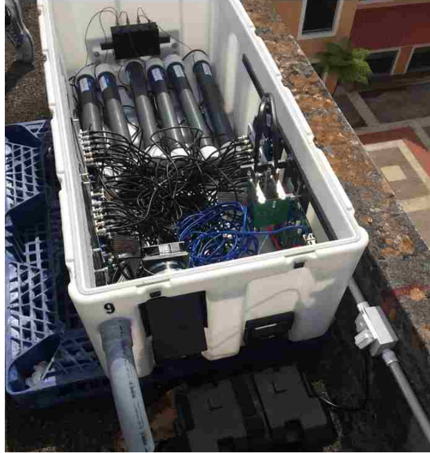
Figure 3.2. The interior of a fully assembled TETRA-II box. The six BGO are seen at the top, with the electronics at the opposite end. Each box is roughly 160 \times 70 \times 80 cm.
