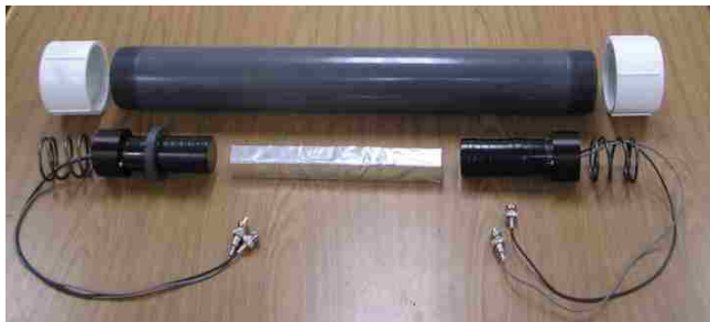
Figure 3.1. The PVC assembly containing a BGO crystal viewed by 2 PMTs. The system is spring mounted with a PVC tube with PVC collars to support the BGO and PMTs.
