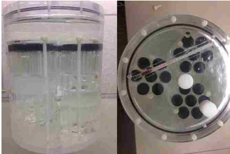
Figure 2.2: The Data Spectrum Corporation's MRI phantom. The phantom includes inserts for spatial resolution, slice thickness, slice profile, linearity, and quantitative imaging (left), though only the quantitative imaging insert (right) is of interest to this study.
