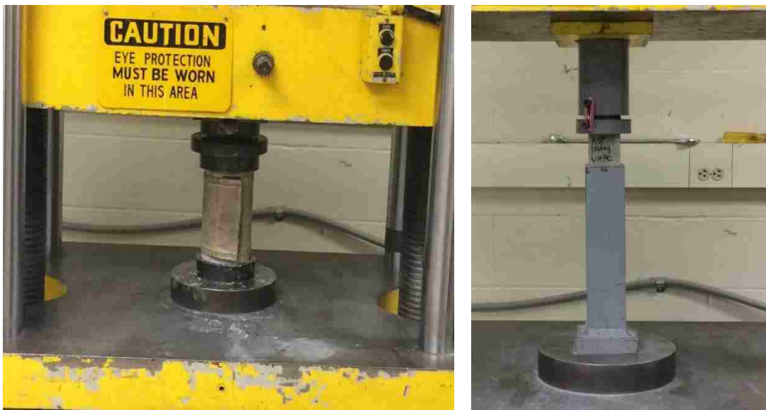
Figure 5.17 Testing cylinder and cube in Tinius Olsen
