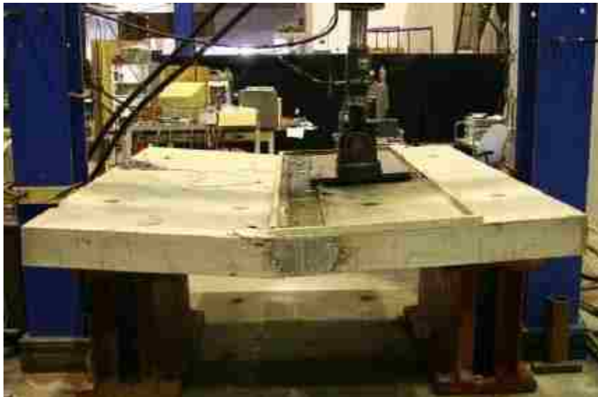
Figure 2.9 Specimen after failure in FHWA study HRT-11-023
