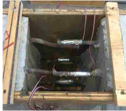
Figure 3.6 Anchored rebar detail
