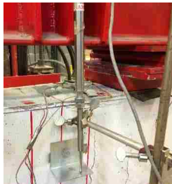
Figure 5.9 LVDT at midspan
