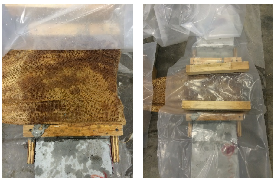
Figure 5.20 Curing using burlap
