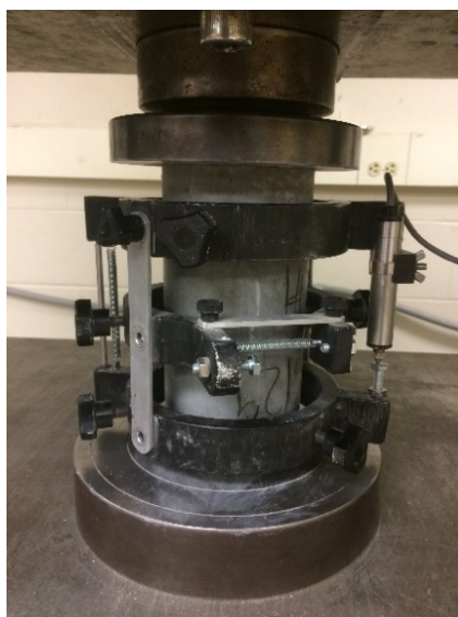
Figure 5.19 Modulus of elasticity testing
