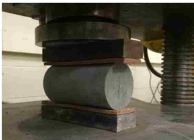
Figure 5.18 Splitting tensile test on UHPC specimen
