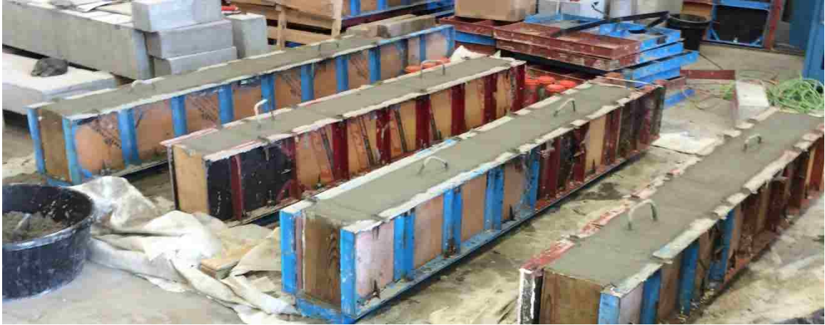
Figure 5.2 Control specimens after casting
