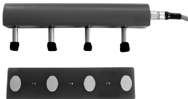
Figure 3.8. Electrical resistivity measurement (Proceq SA 2007)
