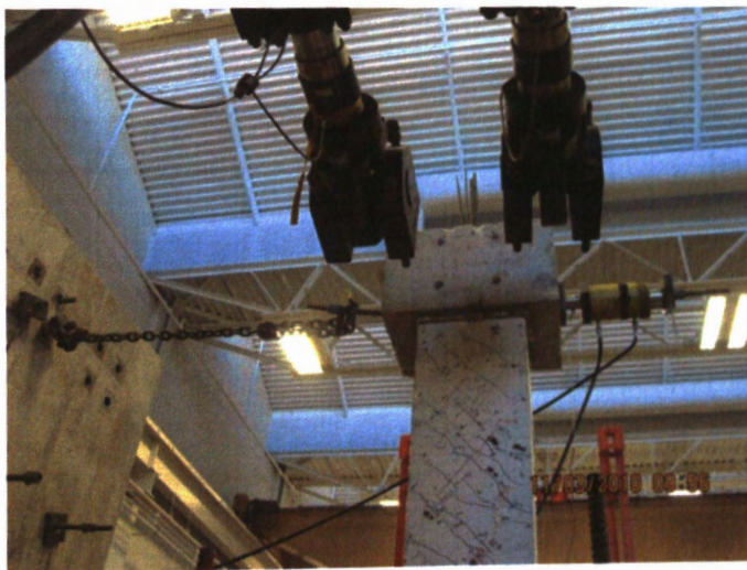
Figure 4.15. Column Straightening Setup For Columns #2 and #3
