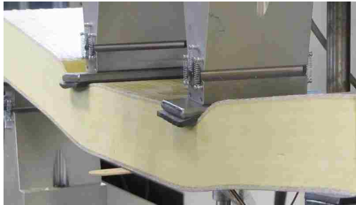
Figure 5.27: Four Point Flexural Testing Ultimate Failure Due to Excessive Local Indentation for Type 1
