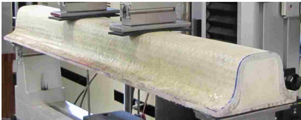
Figure 5.21: Four Point Flexural Test Specimen for Type 3
