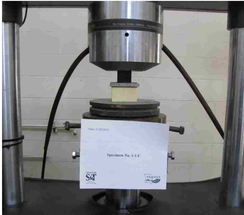
Figure 4.3: Flatwise Compression Testing Setup
