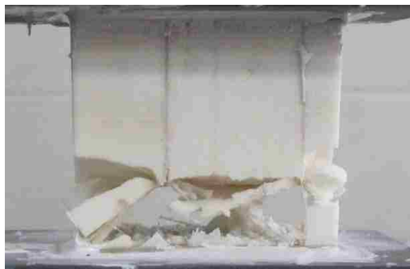
Figure 4.22: Damage During Bond Failure for Flatwise Tension Testing on Type 2
