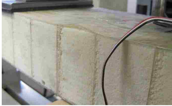
Figure 5.32: Four Point Flexural Testing Initial Failure by Intra-cellular Dimpling of the Top Facing for Type 2
