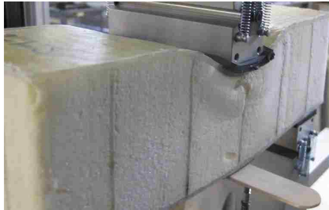
Figure 5.13: Three Point Flexural Testing Ultimate Failure by Fracturing of the Reinforcing Webs and Excessive Local Indentation for Type 2
