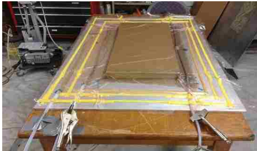
Figure 3.4: VARTM Process for Small Scale Specimens
