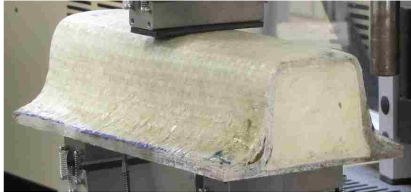
Figure 5.3: Three Point Flexural Test Specimen for Type 3
