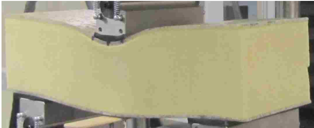
Figure 5.8: Three Point Flexural Testing Ultimate Failure by Excessive Local Indentation for Type 1
