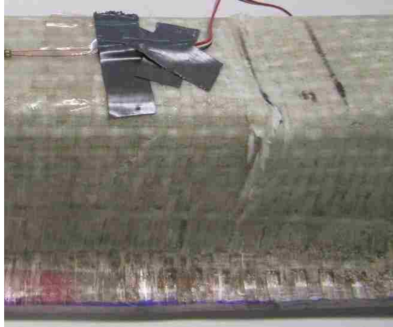
Figure 5.39: Four Point Flexural Testing Fracture Due to Compression Failure of the Top Facing Under the Load Point for Type 3
