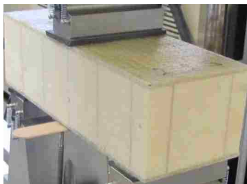
Figure 5.2: Three Point Flexural Test Specimen for Type 2
