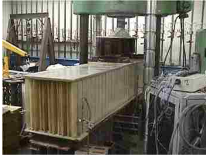
Figure 2.7: Flexural Test of FRPH Panel (Nystrom et al., 2002)
