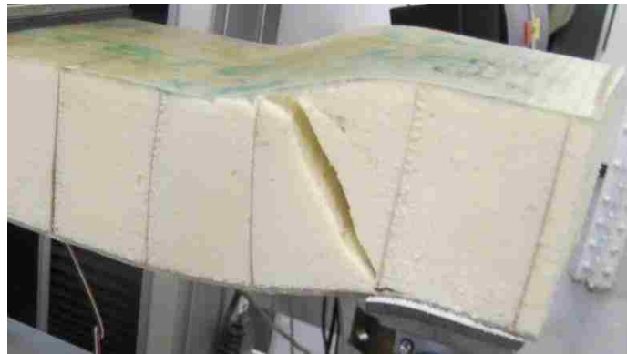
Figure 5.33: Four Point Flexural Testing Ultimate Failure by Shear Fracture in the Core Material for Type 2
