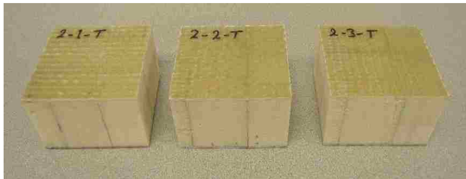
Figure 4.14: Flatwise Tension Testing Specimens for Type 2
