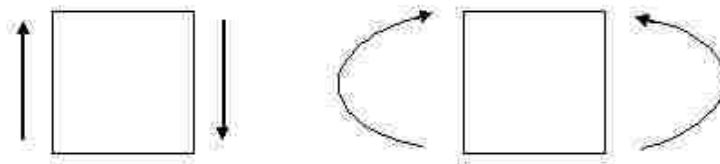
Figure 2.11: Sign Convention for Positive Bending Moments and Shear Forces
