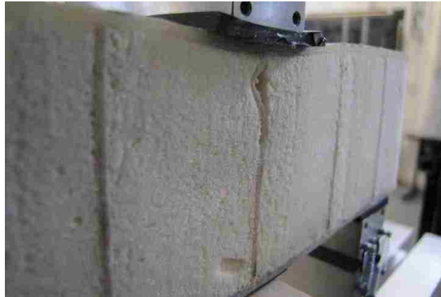
Figure 5.12: Three Point Flexural Testing Initial Failure by Buckling of the Reinforcing Webs and Local Indentation for Type 2
