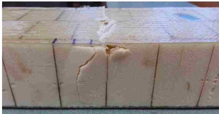
Figure 5.34: Four Point Flexural Testing Ultimate Failure by Compressive Failure of the Top Facing for Type 2
