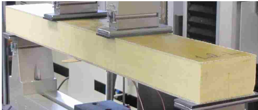
Figure 5.19: Four Point Flexural Test Specimen for Type 1
