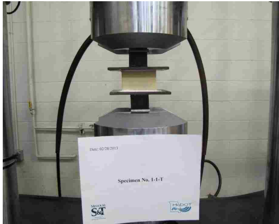
Figure 4.16: Flatwise Tension Testing Setup
