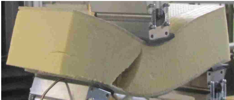
Figure 5.9: Three Point Flexural Testing Ultimate Failure by Shear Fracture in the Core Material for Type 1
