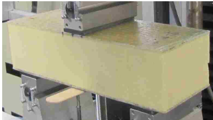
Figure 5.1: Three Point Flexural Test Specimen for Type 1
