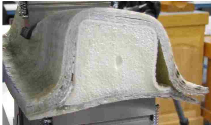
Figure 5.18: Three Point Flexural Testing the Unsymmetrical Deformation Caused by Delamination at the End of the Test for Type 3
