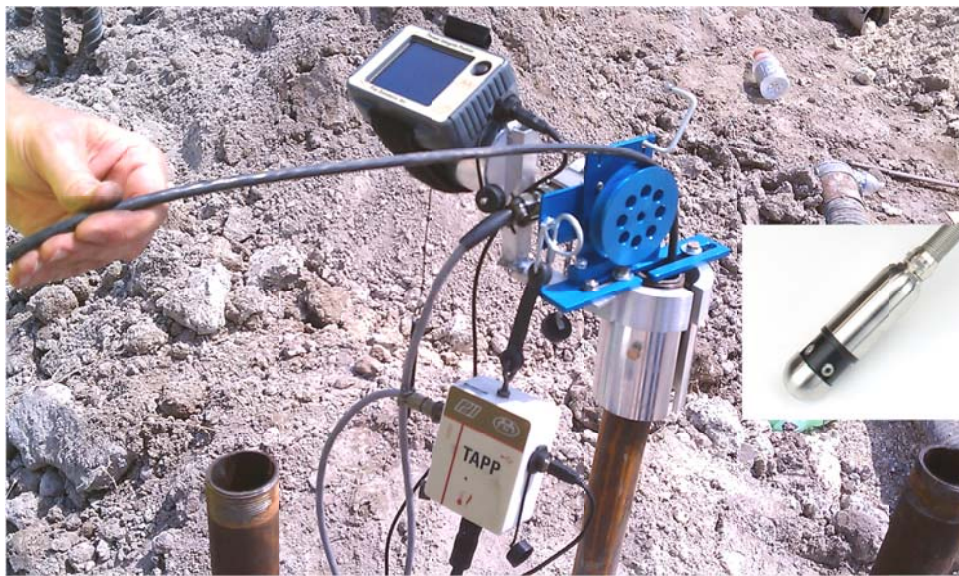
Figure 3.8 Thermal profiling using the thermal probe method (probe shown separately).
