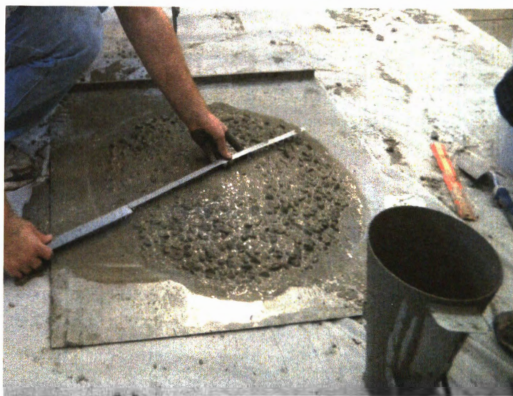
Figure 4.2. Measure Concrete Diameter During Slump Flow Test
