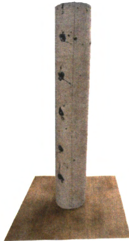
Figure 5.2. Typical Shrinkage Specimen
