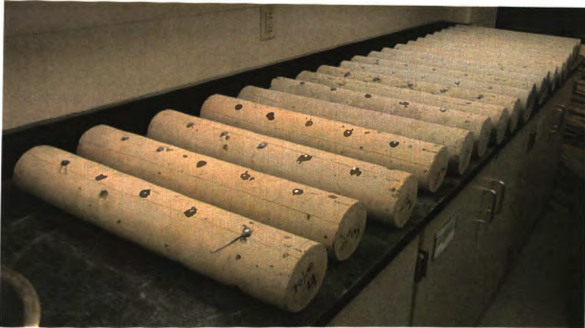
Figure 5.3. Concrete Shrinkage Specimens
