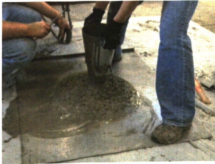
Figure 4.1. Raising the Mold During Slump Flow Test
