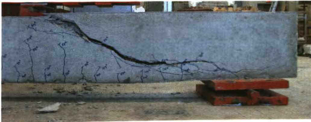
Figure 6.44. Control-NS-2 Beam at Failure
