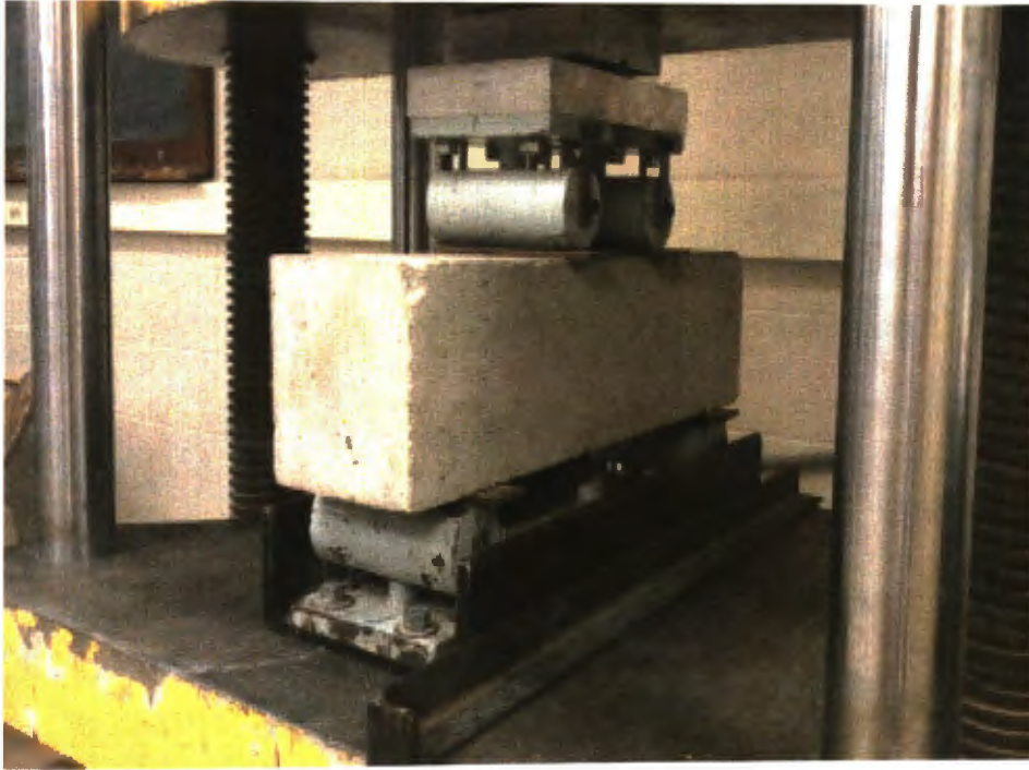
Figure 4.8. Modulus of Rupture
