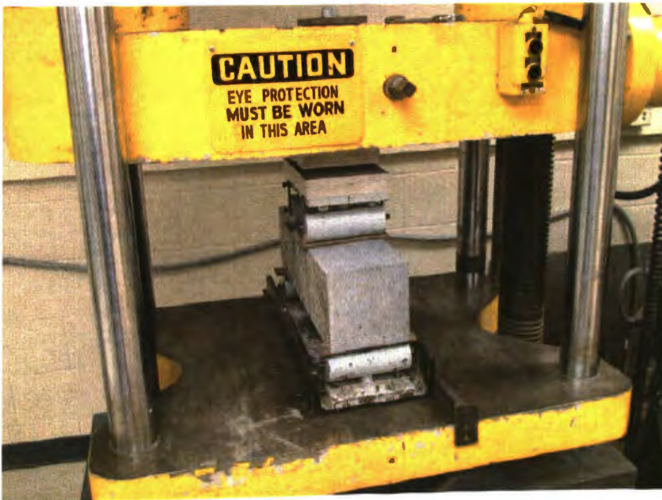
Figure 4.7. Modulus of Rupture
