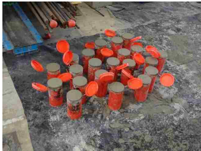
Figure 3.15. Test Girder CIP Deck QC/QA Specimens
