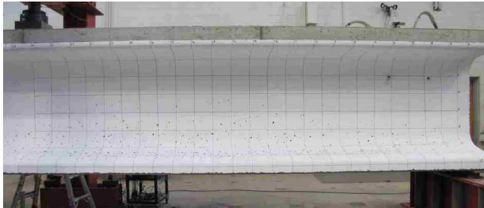
Figure 3.20. Crack Monitoring Grid
