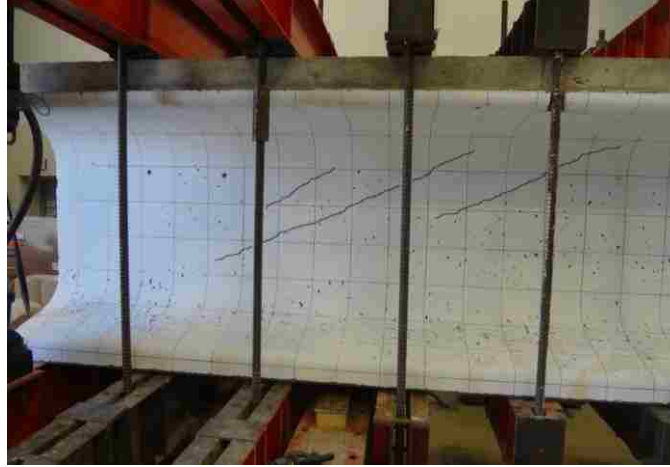
Figure 3.24. Cracks in Non-Tested Region (Cracks traced for clarity)
