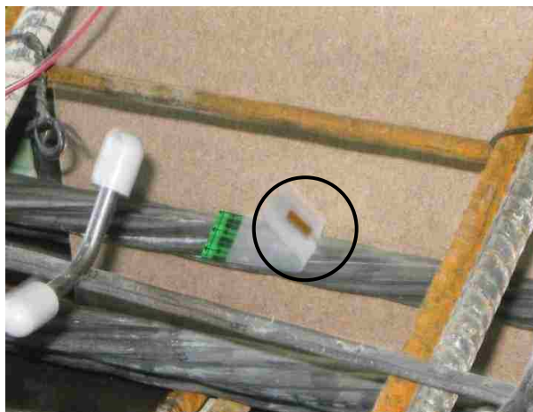
Figure 3.5. Electrical Resistive Strain Gauge
