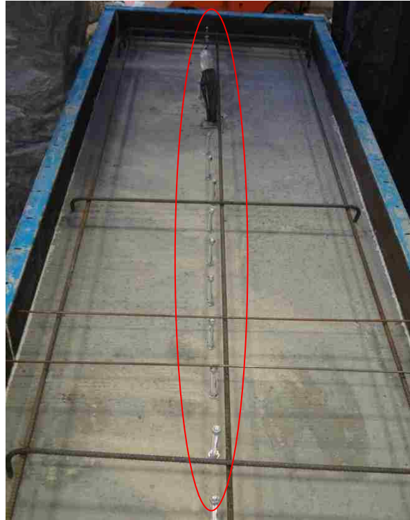
Figure 3.4. Shear Studs in Region 3
