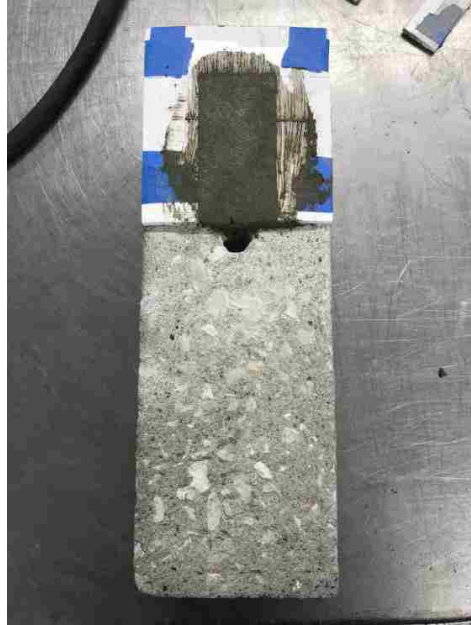
Figure 3.16. Internal matrix layer application for anchorage specimens (100 mm bond length shown, 330 mm bond length similar)
