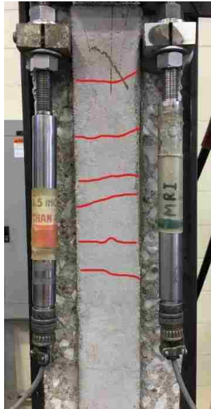
Figure 4.5. Transverse cracking for specimen DS_330_50_C_1 (cracks shown in red)
