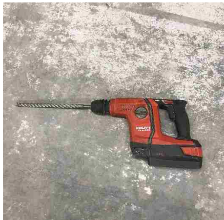
Figure 3.13. Concrete drill used to drill anchor hole into prisms
