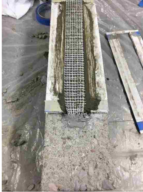
Figure 3.10. Fibers impregnated into internal matrix layer (anchored specimen shown, control specimen similar)
