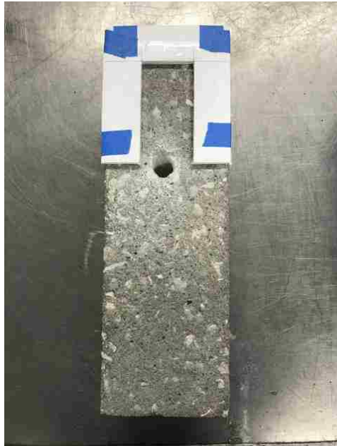
Figure 3.15. Anchorage hole drilled into concrete prism and internal matrix layer form (100 mm bond length shown, 330 mm bond length similar)
