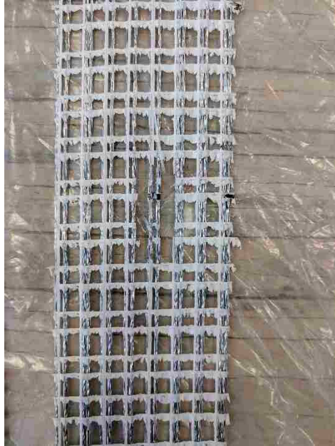
Figure 3.23. Location of strain gauge without fiberglass backing
