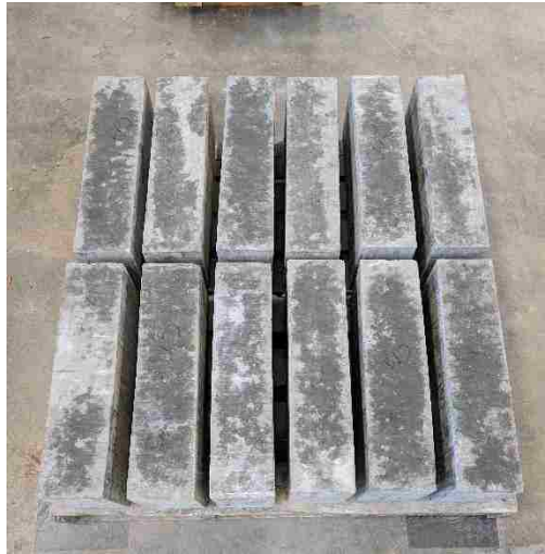
Figure 3.7. Newly cast concrete prisms prior to sandblasting
