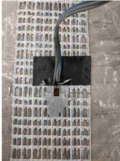
Figure 3.28. Strain gauge with external leads
