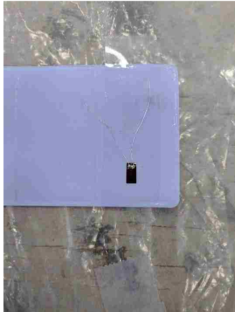
Figure 3.26. Strain gauge prepared for installation
