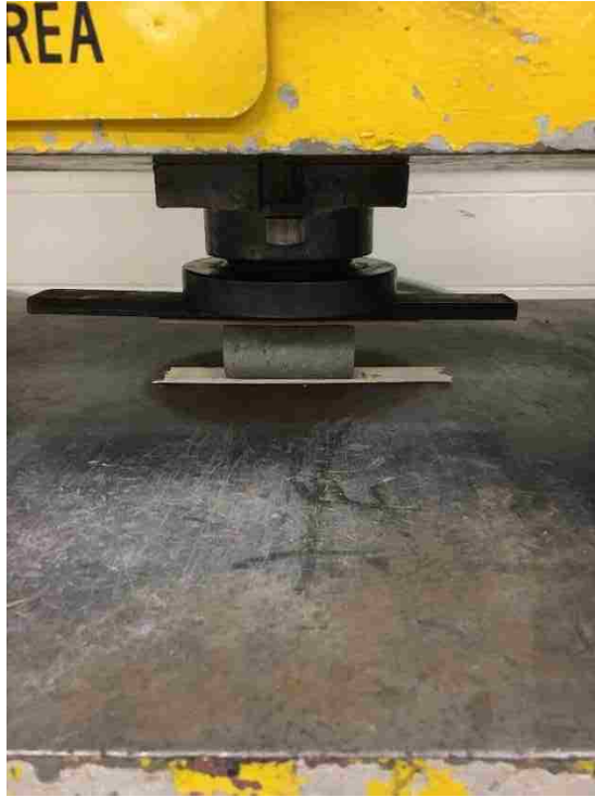
Figure 3.5. Splitting tensile strength test setup
