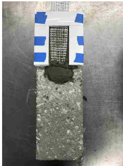
Figure 3.19. External matrix layer form secured onto internal matrix layer form (100 mm bond length shown, 330 mm bond length similar)
