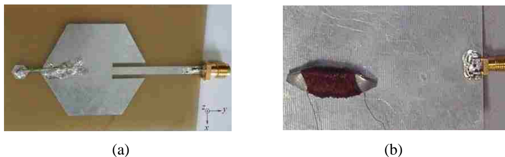
Figure 5.39. Prototype reconfigurable hexagonal patch antenna with reed switch. (a) top view, (b) bottom view [126].
