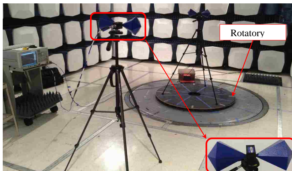
Figure 6.44. Measurement setup to measure pattern of commercially available BicoLOG20300 antenna.
