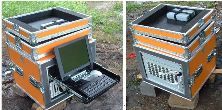
Fig. 7. MST Orange Box. (a) Front of the Orange Box showing the PC interface. (b) Rear panel showing connectors for sensors that include thermocouples, load cells, strain gauges, and LVDT's.
