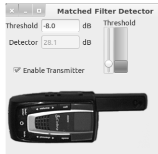
Figure 5.2: The simple GUI for the matched filter detector. The image of the radio receiver indicates that a device has been detected.
